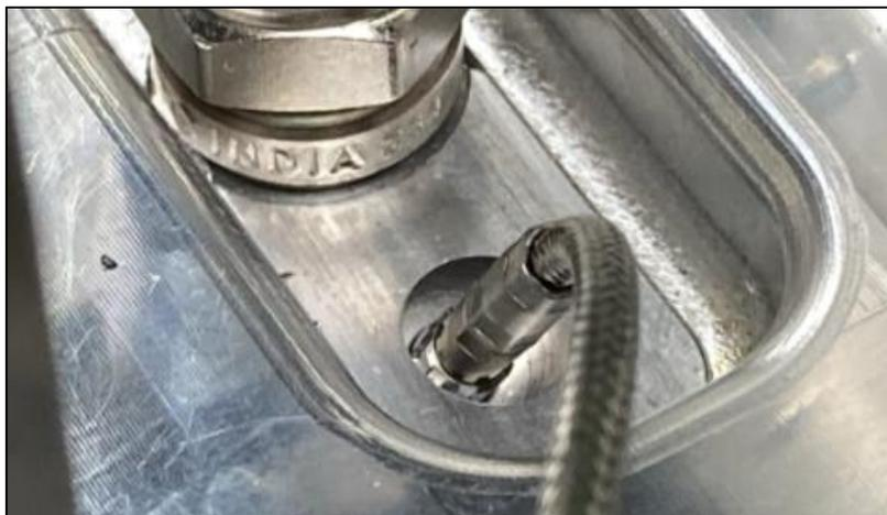
*Figure 44 - Pressure Transducer in Position*
