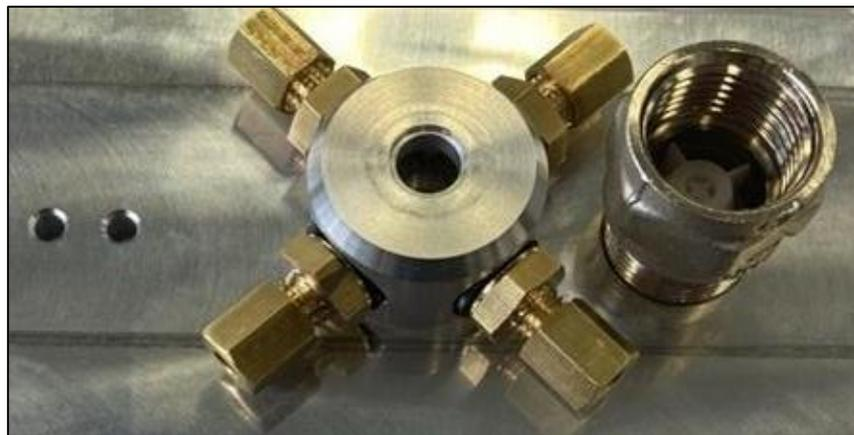
*Figure 53 - Oil Distribution Block and Crankcase Breather in Position on the Front Shaft Housing*
