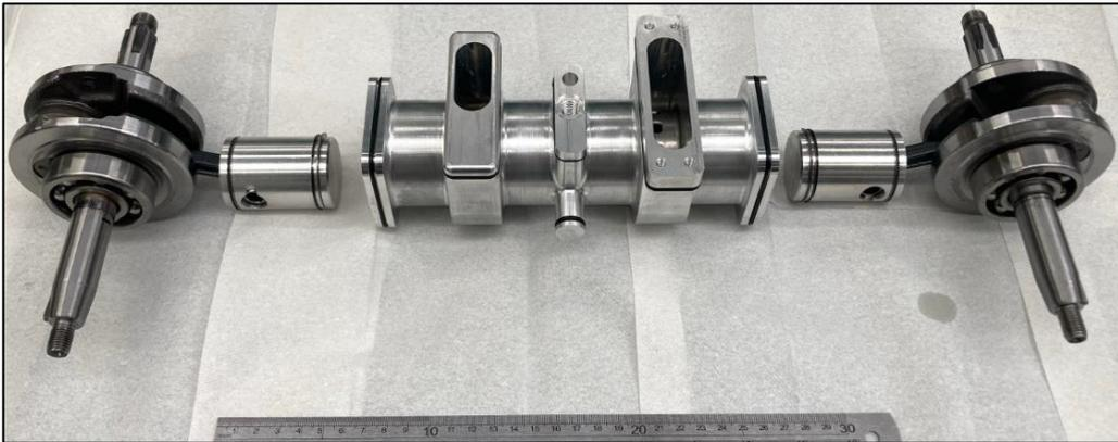
*Figure 129 - Crank Slider Mechanisms and Cylinder Block and Liner Before Assembly*
