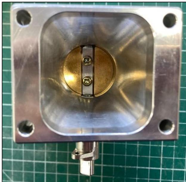
*Figure 139 - Bypass Valve Closed; Bore Diameter Approximately 27 mm*
