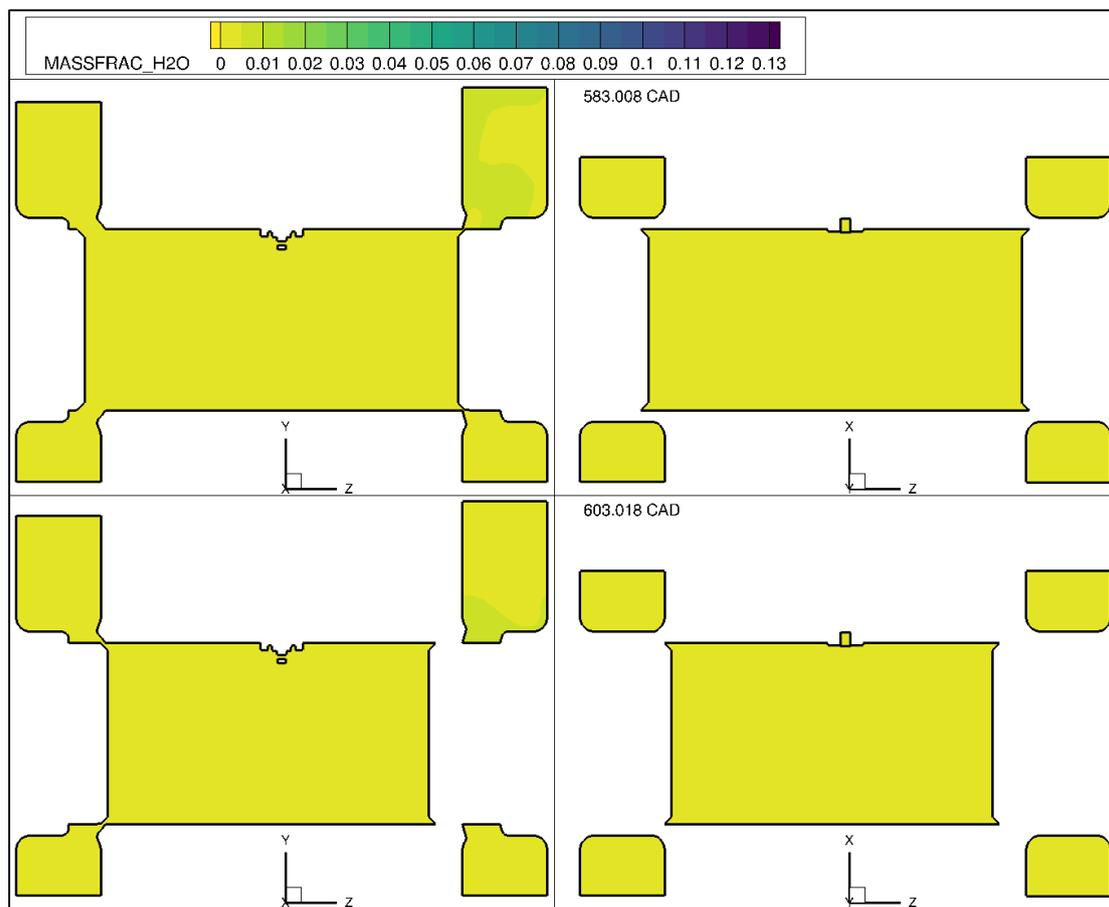
Figure 108 - H<sub>2</sub>O Mass Fraction in the X Plane (Left) and Y Plane (Right), 583 CAD to 603 CAD
