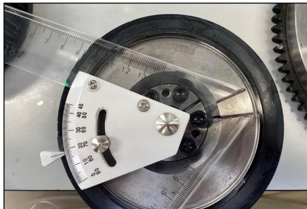
*Figure 114 - Adding Timing Marks to the Crankshaft Pulleys*
