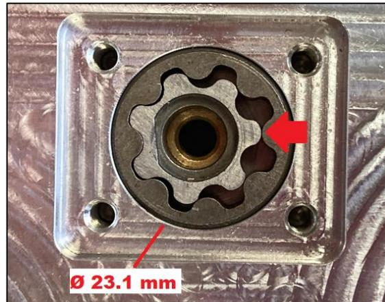
Figure 48 - Oil Pump Parts in Recess in Rear Engine Case
