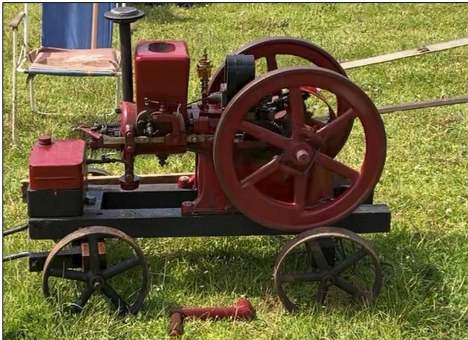
*Figure 4 - Amanco Engine with Mechanical Spark Ignitor - Exhibited at the 2022 Strumpshaw Steam Engine Rally (Exhibitor not Known)*
