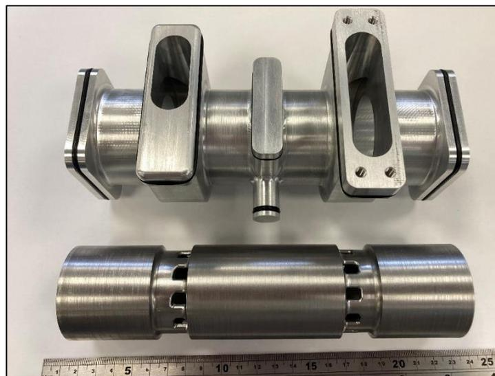
*Figure 33 - Cylinder Block and Liner*
