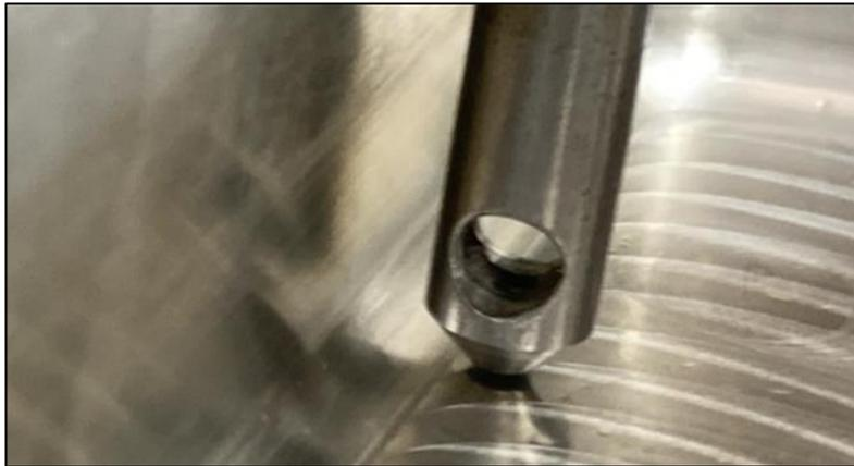
*Figure 51 - Oil Pickup Tube Position*
