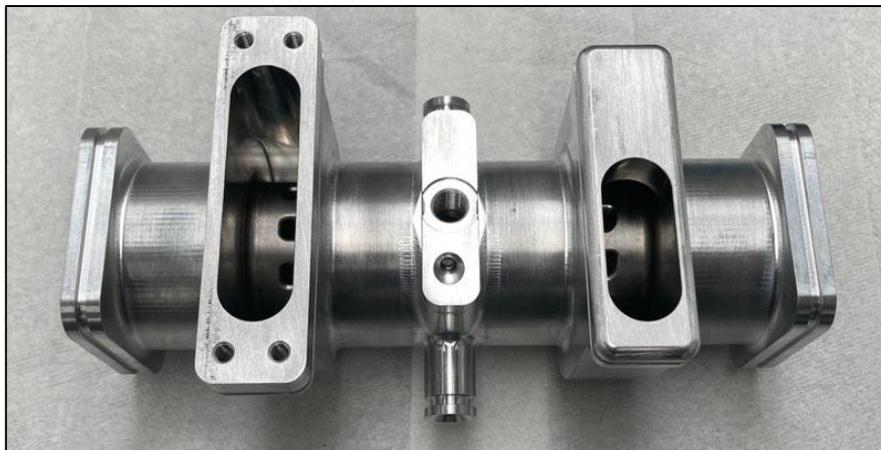
*Figure 126 - Completed Cylinder Block and Liner Assembly, With Spark Plug, Injector and Pressure Transducer Seats, Ready for Installation; Overall Length of Cylinder Block 203 mm*
