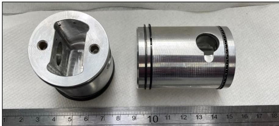
*Figure 32 - Completed Pistons for the New Prototype*
