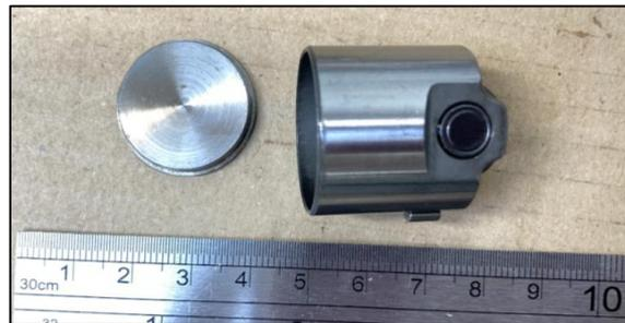
*Figure 58 - GDI Pump Plunger and Steel Pad*
