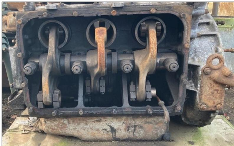
*Figure 16 - Roots TS3 With Rocker Cover Removed*
