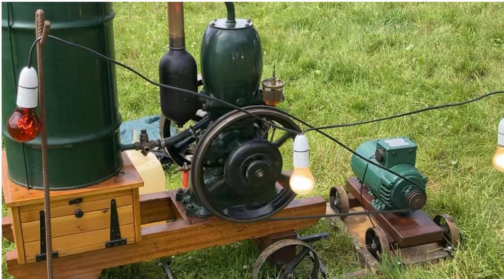
*Figure 7 - Petter Tank Cooled 2 Stroke Engine Lighting some Incandescent Bulbs, exhibited at the 2022 Strumpshaw Steam Engine Rally, Norfolk, England (Exhibitor not Known)*
