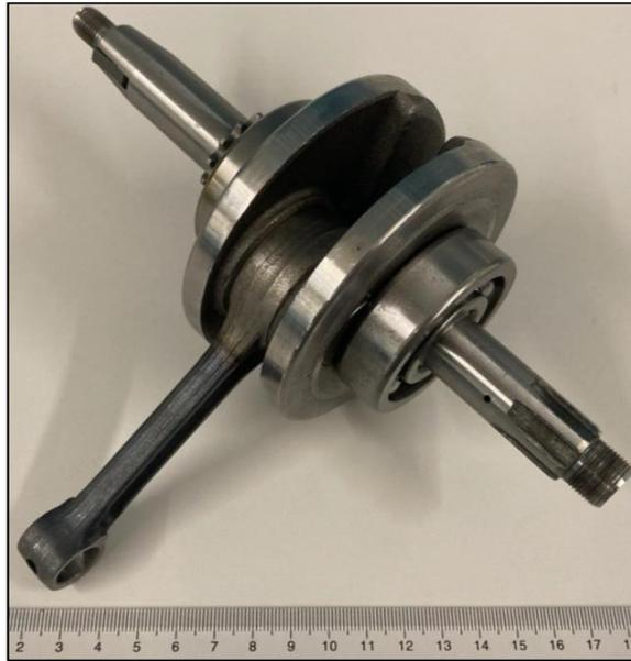
*Figure 29 - One of the Crankshafts for the Engine*
