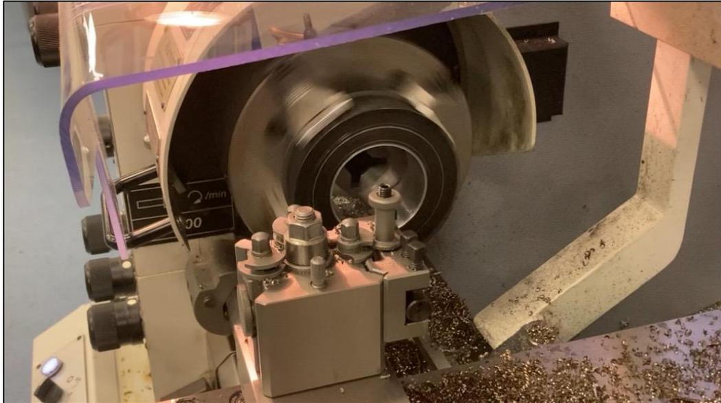
*Figure 133 - Flywheel Pulley during Machining*
