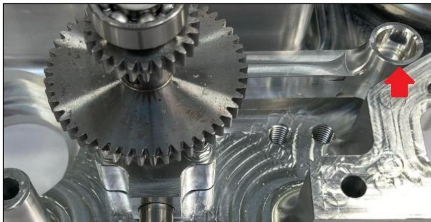
*Figure 52 - Oil Pump in the Rear Engine Case*
