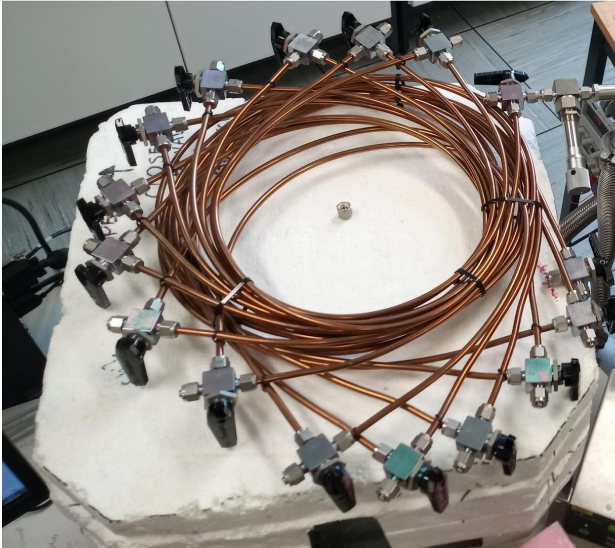
*Figure 4.3. The simple sub-sampler 'Luna'. Note the extensive copper-coloured coils, each loop is a sample loop, attached to a 3-way valve at the exterior of the sub-sampler.*
