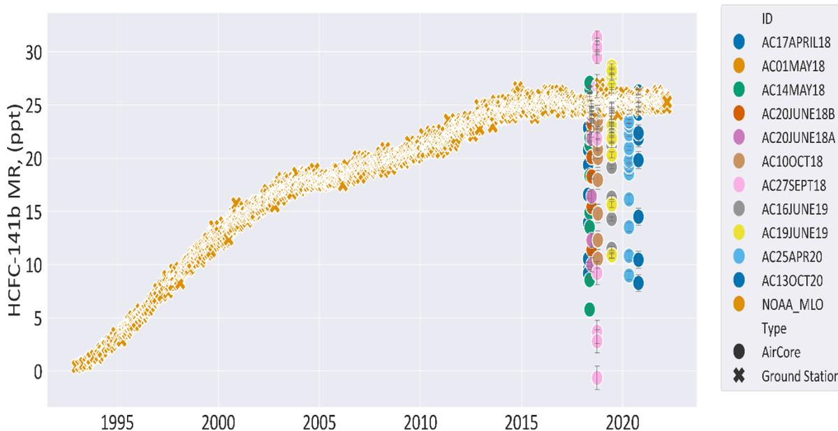
Figure 4.20. Mixing Ratio for HCFC-141b plotted against date (yr), for the AirCore flights examined here, and the NOAA tropospheric trend from Mauna Loa Observatory (MLO). As HCFC-141b has a seasonal cycle a global trend was unsuitable. There are a limited number of observation stations, so MLO was chosen as it was the closest in latitude.
