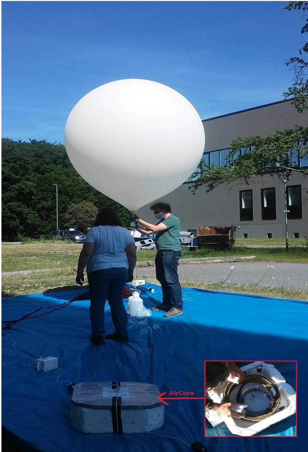
*Figure 2.1. A photograph of an AirCore (polystyrene box in foreground) with an insert showing the AirCore device itself. In the background can be seen the helium balloon being filled.*
