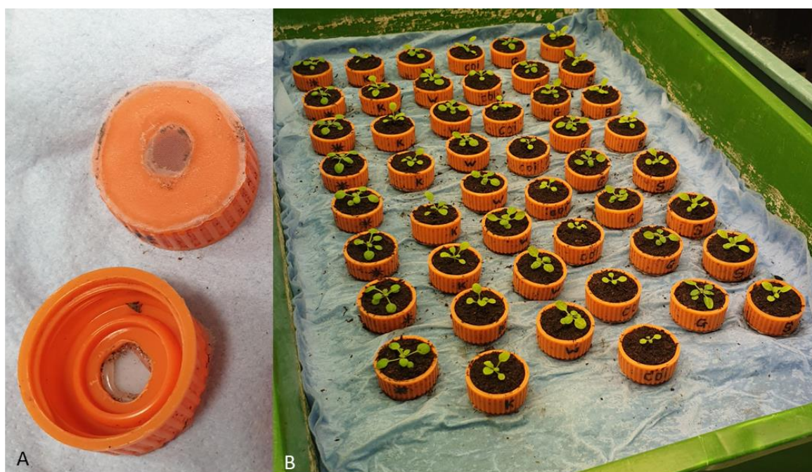
Figure 3.1. A: photograph demonstrating modifications made to 50ml Corning centrifuge tube lids, with holes drilled in the bottom and covered in mesh to allow contact with water and B: photographic example of Arabidopsis seedlings in modified corning tube “pots”, on damp blue roll to allow watering from below.
