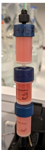
Figure 14. Three StrepTactin columns in series becoming saturated with red material during the loading of spent media, consistent with the expected gene products.
