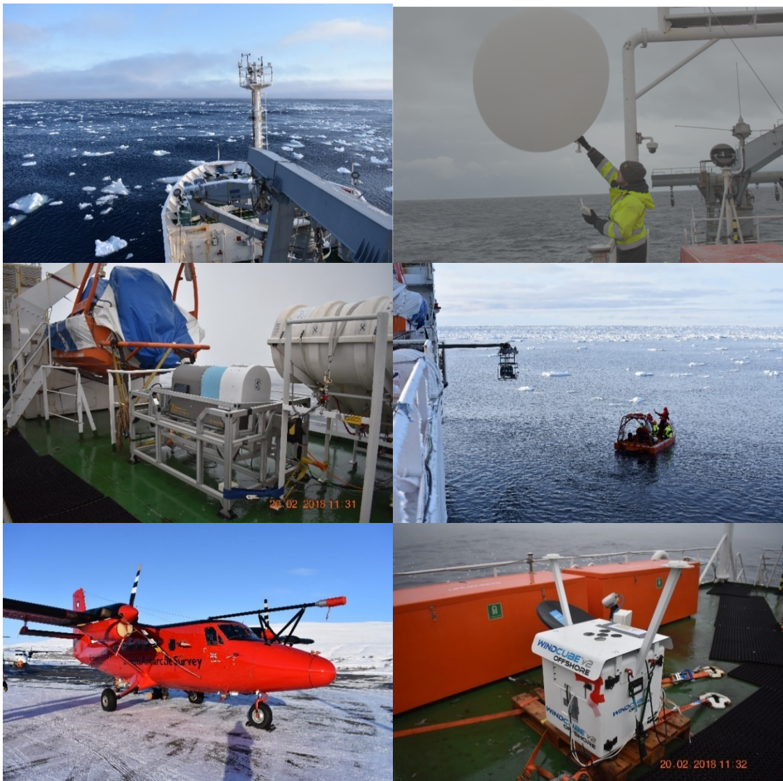
Figure 2.4 Photos of observational equipment used during the Iceland-Greenland Seas Project field campaign: a) the WeatherPack meteorological instruments on the bow mast of the Alliance ; b) a radiosonde launch; c) the RPG Hatpro radiometer; d) a CTD cast being performed; e) the British Antarctic Survey DH6 Twin Otter research aircraft; and f) the Windcube lidar and Micro Rain Radar.
