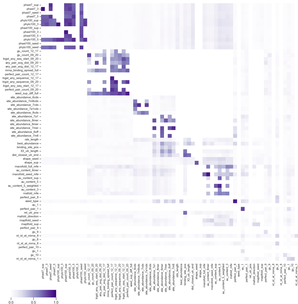
Figure 5.9: Training set feature correlation heatmap. The correlation of each feature pair is compared in a hierarchically clustered heatmap, where a dark colour indicates higher correlation. A number of closely related feature clusters exist, notably those relating to evolutionary conservation and supplementary binding.
