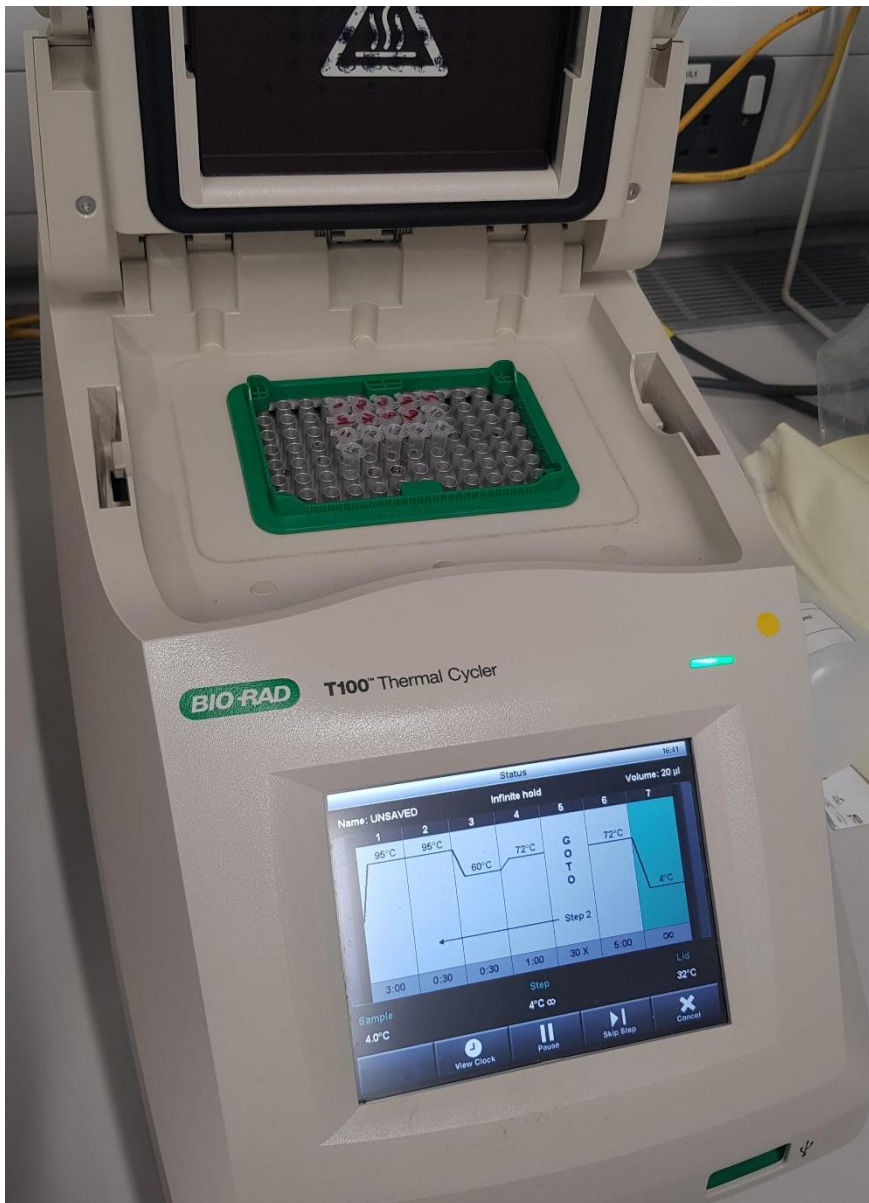
Fig 2.2: Example of PCR tubes being loaded into Thermocycler to undergo cDNA synthesis
