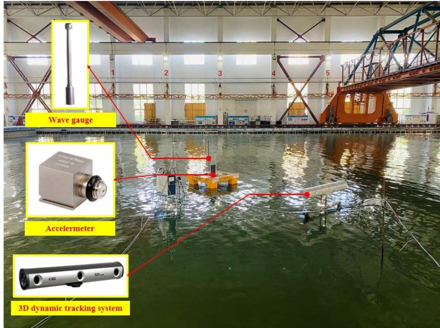
Fig. 14: The physical model of the platform and sensor arrangement.
