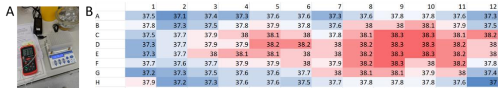
Figure 2.9. Temperature measurement on a 96-sample format using a Bioshake iQ thermomixer set at 37°C. (A) shows the measurement of the temperature, and (B) table shows the temperature results.
