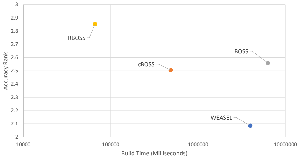
Fig. 4.6 Scatter graph plotting average accuracy rank against build time on a log scale for cBOSS and other dictionary classifiers. Classifiers close to the bottom are more accurate, and those close to the left are faster.
