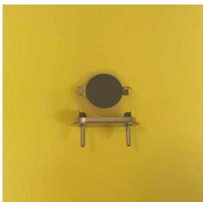
Figure 10.2 b) Photograph of a quartz crystal electrode.
