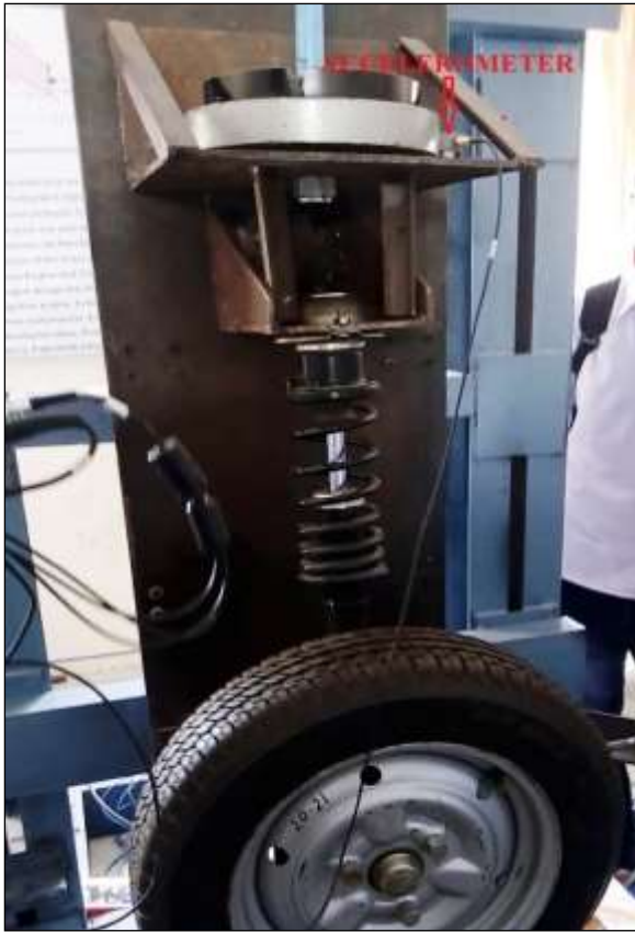
Fig 3: Position of Accelerometers – Sprung Mass Fig 4: Position of Accelerometer – Unsprung Mass
