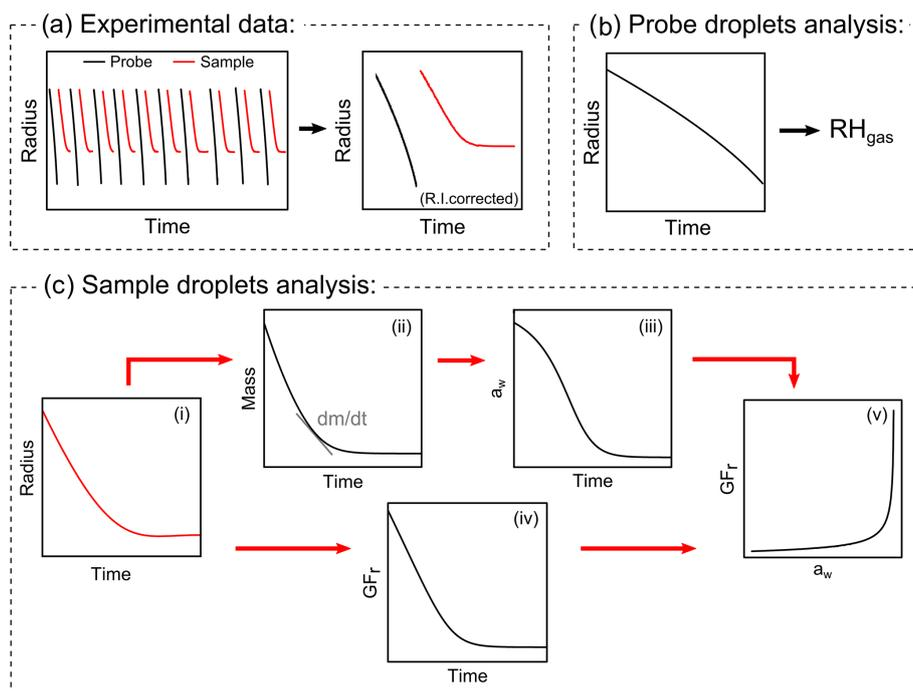
**Figure 1.** Schematics representing the retrieval of hygroscopic growth curves from comparative kinetics experiments in a CK-EDB. An experimental sequence of alternating single evaporating probe and sample droplets is collected (a). For each pair of probe and sample droplets, the gas phase RH is inferred from the evaporation kinetics of the probe (b) and this information is used to analyse the corresponding sample droplet hygroscopic properties as indicated in (c).
