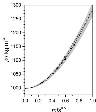
**Figure 9.** DMAS density ( $\rho$ ) dependence on mass fraction ( $\text{mfs}^{0.5}$ ) of solute. Symbols: black squares – measured densities, this work; solid line – third-order polynomial fit of measured  $\rho$  values; grey shaded area – evaluated uncertainty of the density parameterisation (calculated as discussed in the main text); open circles – measured densities from Clegg et al. (2013); dashed line – densities from the apparent molar volumes fitting by Clegg et al. (2013).
