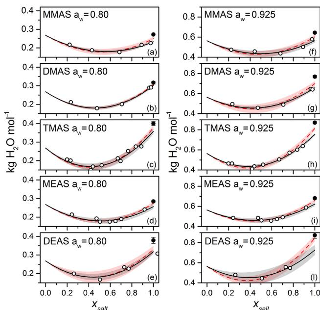
**Figure 7.** Mass of  $\text{H}_2\text{O}$  (kg) per mole of solute as a function of the degree of neutralisation of sulfuric acid by amine ( $x_{\text{salt}}$ ). Symbols: solid circles – data from this work; open circles – data from Sauerwein et al. (2015). Lines: black – ZSR fitting of the data in Sauerwein et al. (2015); red dashed – same ZSR fitting but including the CK-EKB data point for each  $a_w$ ; shaded envelopes – uncertainty associated with the fitting.
