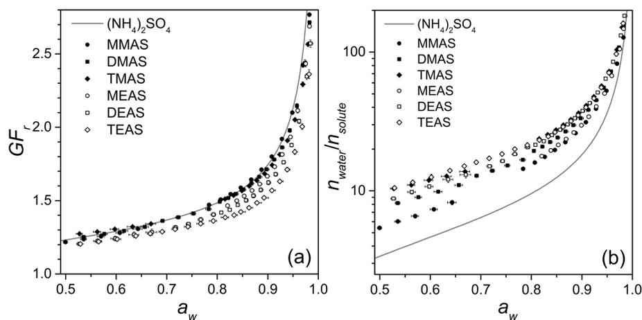
**Figure 3.** Aminium sulfate  $GF_r$  vs.  $a_w$  (a) and  $n_{\text{water}}/n_{\text{solute}}$  vs.  $a_w$  (b) hygroscopic growth plots from CK-EDB experiments. Symbols: ● – MMAS; ■ – DMAS; ◆ – TMAS; ○ – MEAS; □ – DEAS; ◇ – TEAS; line – E-AIM model calculation for  $(\text{NH}_4)_2\text{SO}_4$ . Note that only E-AIM predictions for  $(\text{NH}_4)_2\text{SO}_4$  are reported in this and subsequent figures with the CK-EDB measurements and the E-AIM model compared in Fig. 2.
