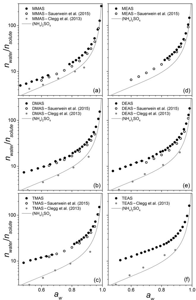
**Figure 5.**  $n_{\text{water}}/n_{\text{solute}}$  vs.  $a_w$  plots for the six aminium sulfates. Symbols: black circles – CK-EDB comparative kinetics measurements; open circles – Sauerwein et al. (2015); grey dots – Clegg et al. (2013) (based on measurements from Qiu and Zhang, 2012); line –  $(\text{NH}_4)_2\text{SO}_4$  calculation from E-AIM model.
