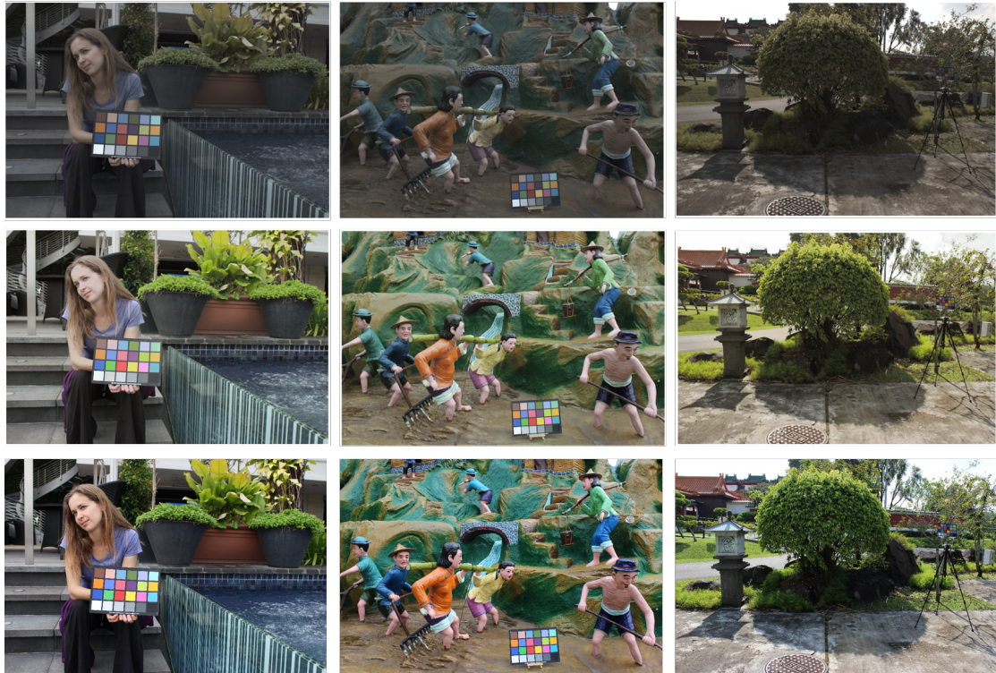
FIGURE 7.4: Examples of raw to JPG transformation using the calibrated lattice: The first row are the raw white balanced images by the shades of grey algorithm. The second row are the results of applied lattice. The last row are the actual JPG outputs from the camera (with the camera's properly white balanced algorithm).
