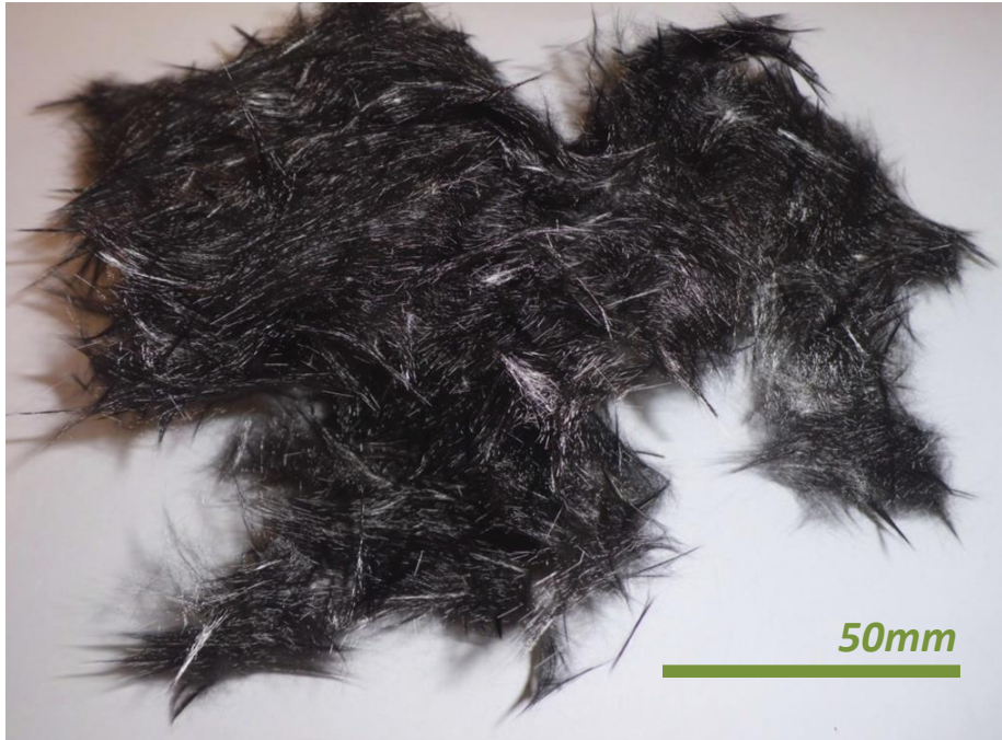
Figure 6 Recycled fibre raw form showing fluffy, discontinuous, 3D random & highly entangled structure
