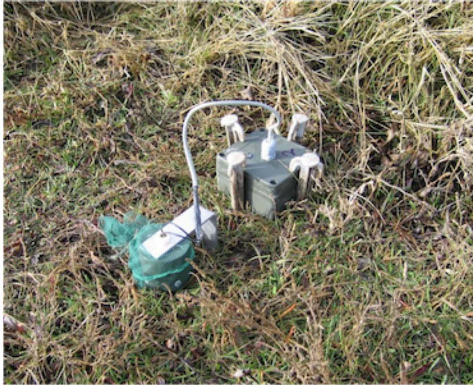
Figure 3.3. The tide gauge installed on the upper marsh at Stiffkey comprising of an event datalogger attached to a float switch which measures the time and duration of tidal flooding. The netting on the float switch case is to prevent fouling by Hydrobia molluscs.
