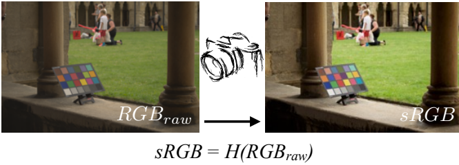
Fig. 2. Color correction (mapping raw to display sRGB) is an homography problem. This figure is also a color chart example which was used for our color correction evaluation.
