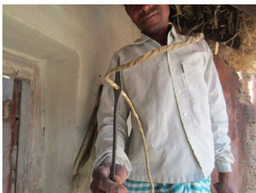
Figure 4-34: Needle used for tying thatch to the battens below
