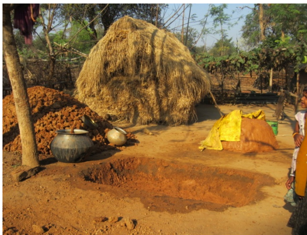
Figure 4-36: Pit dug in the ground for soaking murrum mati , which is used for making khapra
