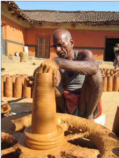
Figure 4-42: Cylinders being shaped on the wheel in the desired size of the final tile
