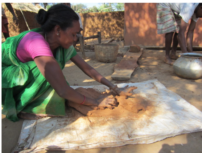
Figure 4-40: A final round of kneading is done by hand
