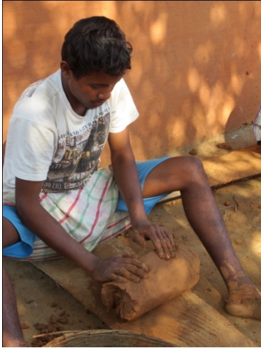
Figure 4-41: The prepared murrum mati is shaped into cylinders before being handed to the potter for shaping on the wheel
