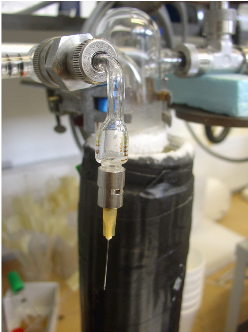
Figure 26: Needle connected to the extraction line via glass tube with Luer-Lock connection
