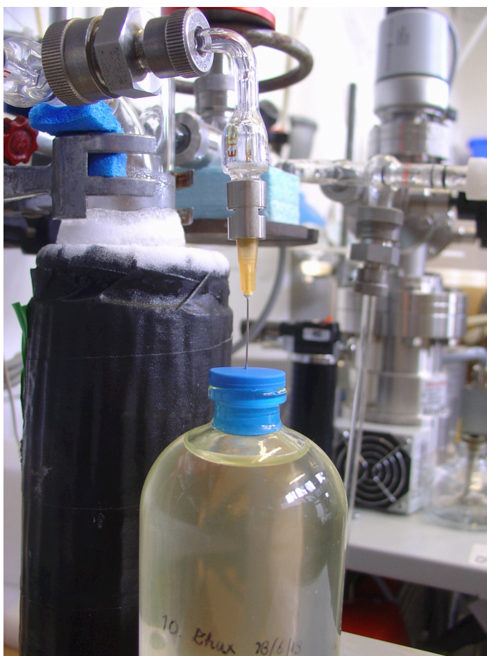
Figure 27: Picture of the extraction line, just prior to sampling. The needle tip is sealed in the stopper of the sample bottle.
