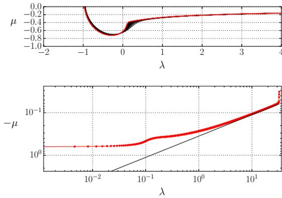
**Fig. 2** Top panel evolution of the free surface during the time-marching procedure (black lines). The grey line (red in the online version) corresponds to the last time step. Notice how the surface has nearly converged, except at the corner near  $(\lambda \approx 0.1, \mu \approx -0.4)$ . Bottom panel converged free surface in the far field. The black thin line represents the asymptotic expression  $h(\lambda) \sim -1/\sqrt{8\lambda}$ . (Color figure online)
