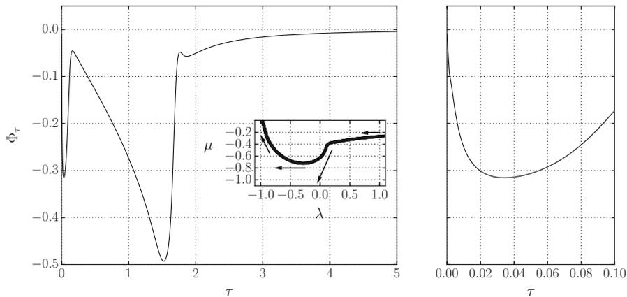
**Fig. 4** Tangential velocity along the free surface corresponding to the last time step. The inset shows qualitatively the direction and modulus of the velocity. The right panel shows close up of the region close to the contact
