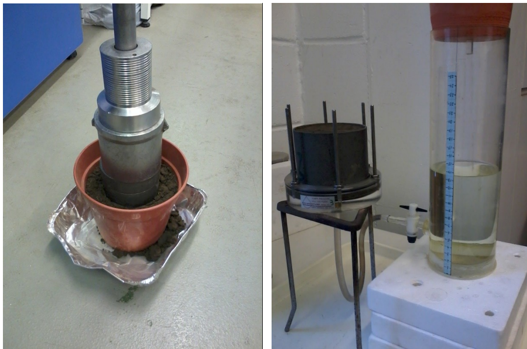
Figure 5.2 SHC experiment: (a: left-hand side) using a field soil corer to remove a sample core from a pot; (b: right-hand side) saturating the core, in a Tempe cell, with 0.01 M \text{CaCl}_2 from the MB. Initially the height of the liquid is just above the base of the cell to ensure gradual saturation by capillary action, minimising the introduction of air bubbles.
