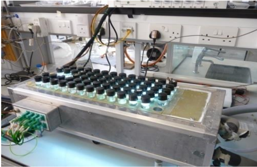
Figure 3. 2 Temperature gradient bar with the insulated cover removed, photo by Sian Foch-Gatrell.
