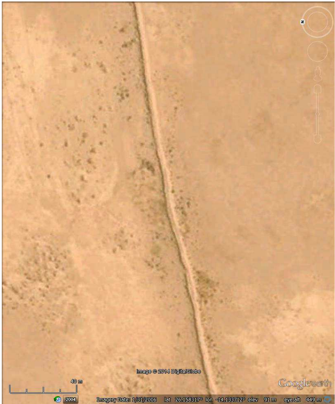
Fig. 4.30: A Google Earth image showing a section of Berm No.1 (in rectangle 215 of Fig. 4.6). When looked at closely, the top of the embankment appears to be flat or slightly indented, perhaps with two ridges. North is to the left of the image. Scale bar at lower left indicates 40 metres. Image date 31/1/06, DigitalGlobe.
