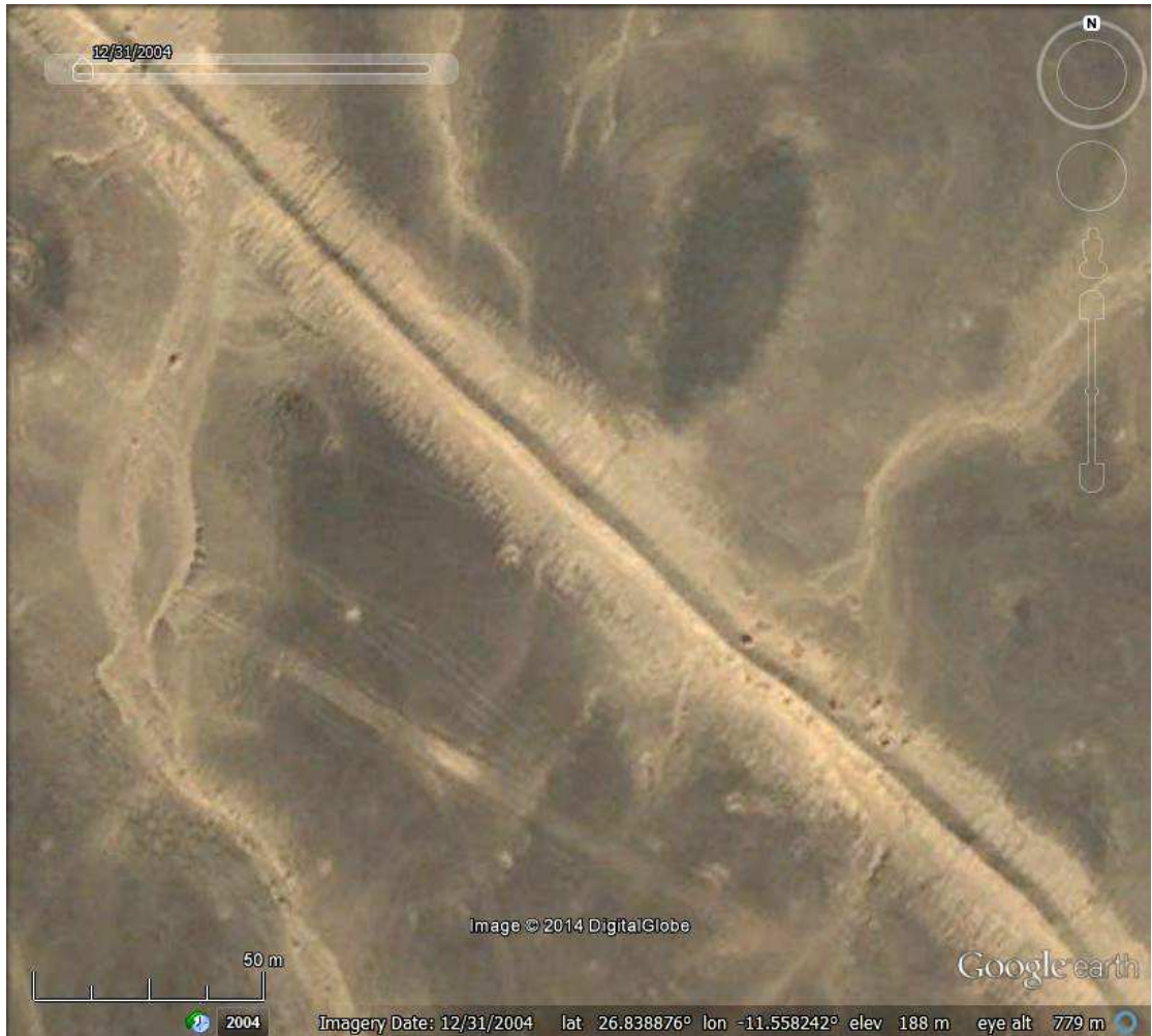
Fig. 4.31: Part of Berm No.1 shown on Google Earth (in rectangle 124 of Fig. 4.6). It is a single embankment with clear evidence of being created by bulldozing from both sides. The top, in places, appears slightly flat, or with a slight depression. Scale bar at lower left indicates 50 metres. Image date 31/12/04, DigitalGlobe.
