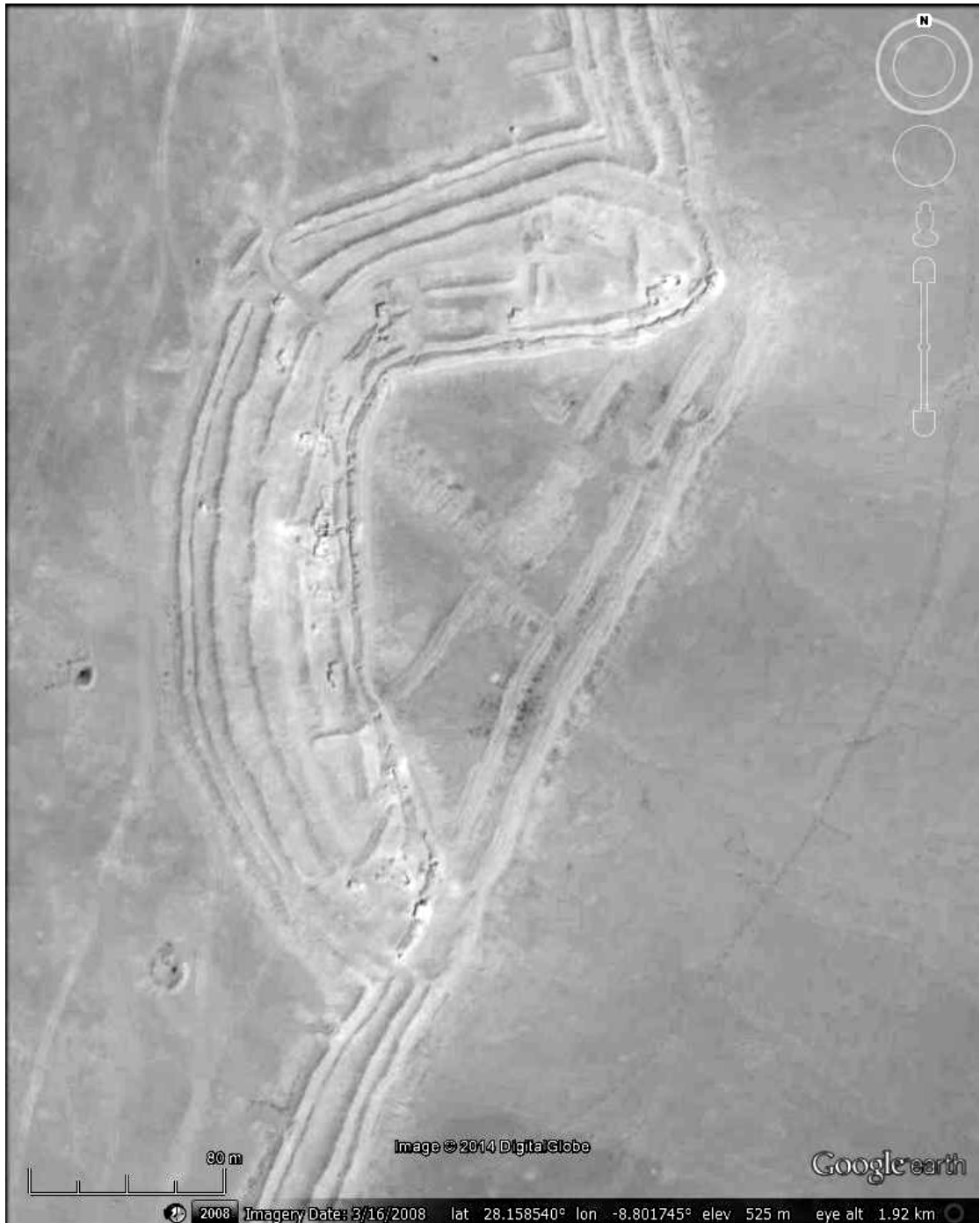
Fig. 4.54: Google Earth image (in monochrome to highlight features) of an irregular shaped fort (ft 1269) on Berm No. 4 (located in rectangle 952 of Fig. 4.6). It used to be a concentric semi-circle but its frontage has been removed and it is now an irregular arc shaped installation. It is sub-divided and there are bunkers. Fighting positions are visible along the east facing front. A cordon of barbed wire is also just visible, about 100 metres in front of the fort, to the east. The scale bar in the lower left indicates 80 metres. Image date 16/3/08, DigitalGlobe.
