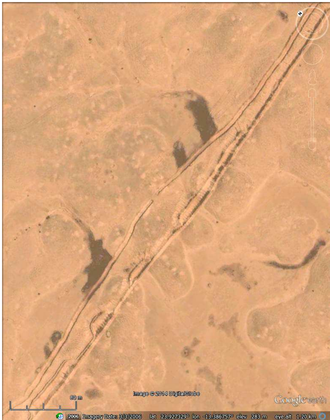
Fig. 4.35: At just to the west of rectangle 491 in Fig. 4.6, this Google Earth image of Berm No.5 clearly shows a frontal defensive bank with subsidiary, intermediate banks. The tracks of the bulldozers which created the embankments are also clearly visible. The second, rear bank is not parallel with the frontal bank, but it also has a ditch on its south side (north is to the top left of the image). A causeway through the second bank and ditch is clearly visible, and water has backed up behind the second barrier, illustrating how the construction of the berms can affect natural drainage. Scale bar at lower left indicates 80 metres. Image date 3/3/06, DigitalGlobe.
