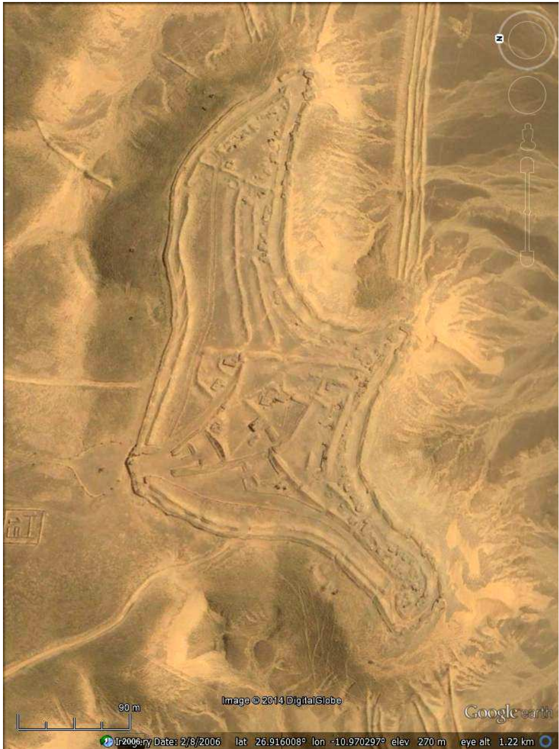
Fig. 4.51: Google Earth image of an irregular shaped fort (ft 681) on Berm No.3 (located in rectangle 126 of Fig. 4.6). Its defensive banks are concentric and follow the natural contours of three spurs of high ground. There are multiple sub-divisions with blast barriers. Buildings and bunkers are spread through out the fort, and there are bunkers and fighting positions at the salients facing south (north is to the left). The scale bar in the lower left indicates 90 metres. Image date 8/2/06, DigitalGlobe.
