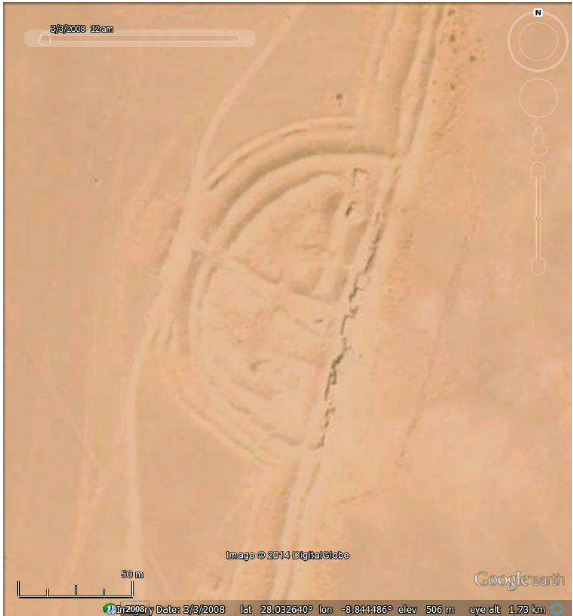
Fig. 4.46: Google Earth image of a semi-circular fortlet (flt 1252) on Berm No.4 (located in rectangle 952 of Fig. 4.6). There are obvious bunkers along the front of the installation facing east. It is also sub-divided with embanked partitions. There is a cordon of barbed wire just in front of the fortlet, which is just barely visible. The scale bar in the lower left indicates 50 metres. Image date 3/3/08, DigitalGlobe.
