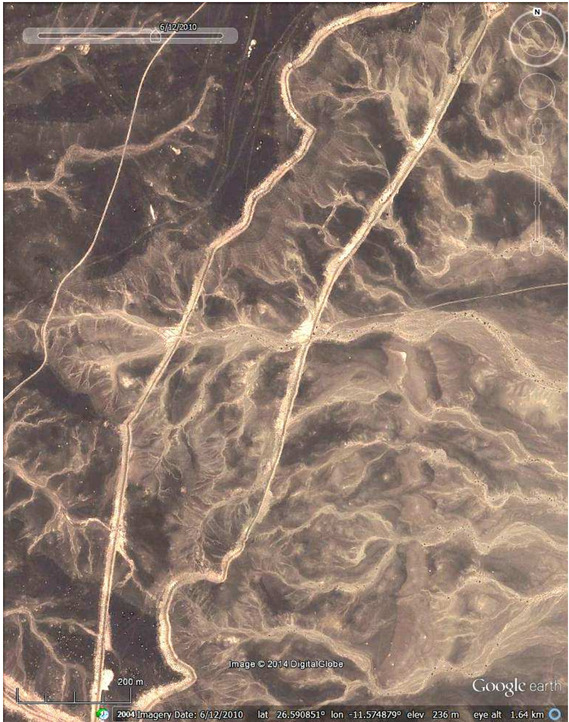
Fig. 4.33: A Google Earth image showing part of Berm No.1 (between rectangles 124 and 157 of Fig. 4.6). It shows the direction of bulldozing in the construction of the barriers (only from one side), and illustrates how the secondary, western barrier more or less follows natural contours, with the primary frontal barrier cutting across natural drainage. A mural track is visible to the west. Scale bar at lower left indicates 200 metres. Image date 12/6/10, DigitalGlobe.
