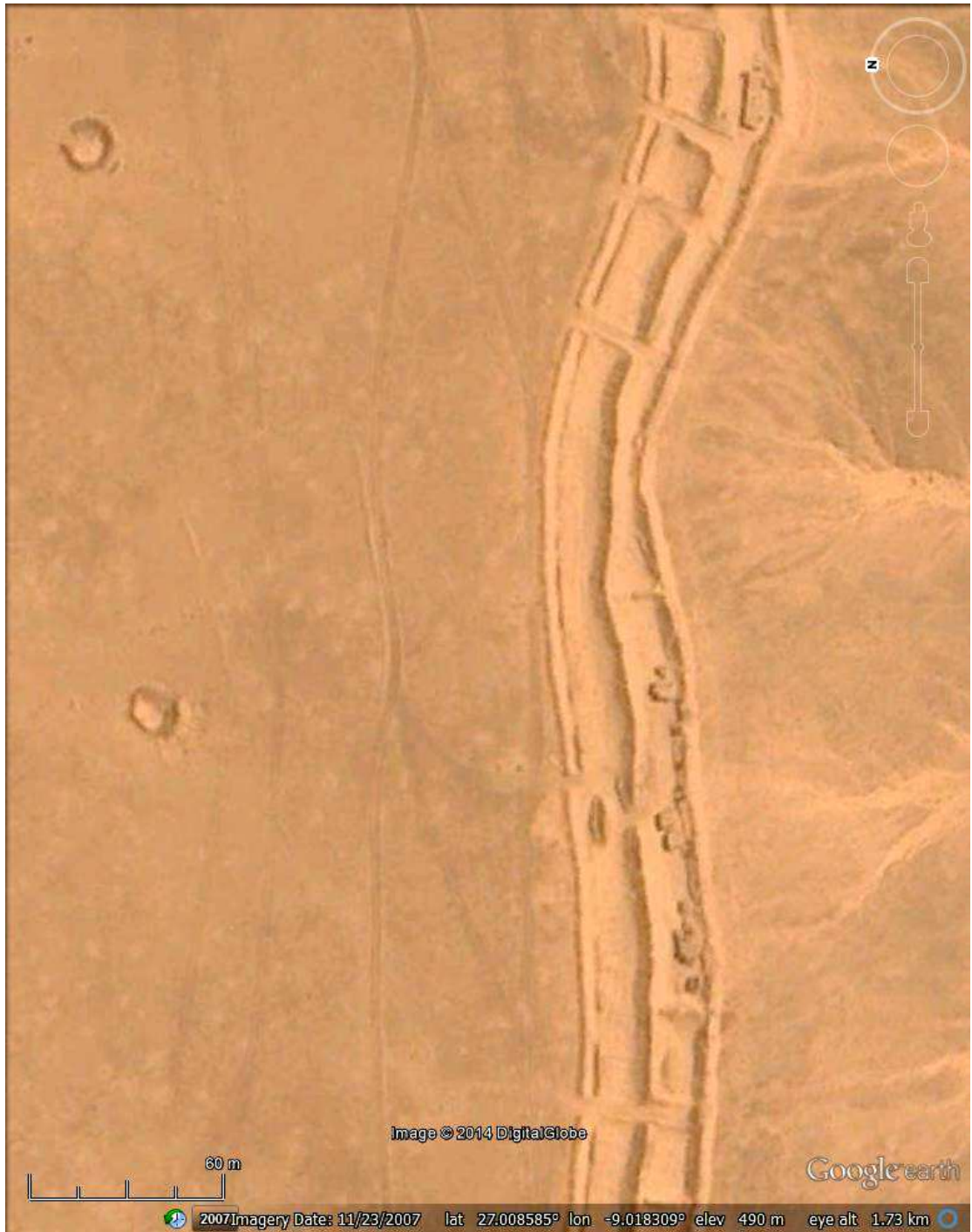
Fig. 4.37: A very good Google Earth image of a short section of Berm No. 4, located in rectangle 100 of Fig. 4.6. It shows a triple embanked barrier, facing south (north is to the left), and positioned on a watershed. A light line in front of the barrier probably represents barbed wire. There are bunker type structures associated with the front embankment. The bank making up the rear of the barrier includes a ditch along its southern side. The earthworks to the north (the left) are probably gun emplacements. The scale bar at lower left indicates 60 metres. Image date 23/11/07, DigitalGlobe.
