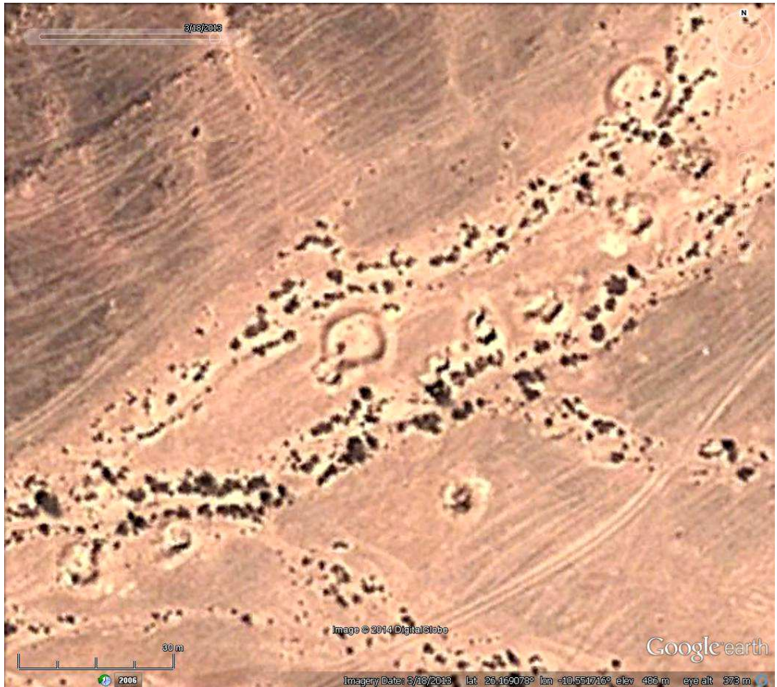
Fig. 6.57: Moroccan defences at Tifariti. A Google Earth view of gun pits in a wadi within the Tifariti box. The pit in the centre, and the two smaller ones in the lower left, have nib-like extensions that represent crew or ammunition bunkers, or protective embankments. There are other dug out features clearly visible as well. The scale in the lower left indicates 30 metres. Date of image: 18/3/13, DigitalGlobe.
