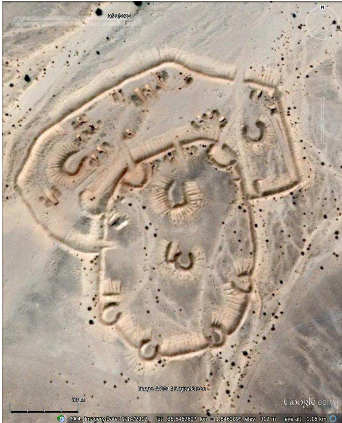
Fig. 4.72: Google Earth image of a redundant, complex firebase (fsb 237) behind Berm No. 1 (located in rectangle 157 of Fig. 4.6). This installation has numerous gun pits and vehicular slots. The scale bar in the lower left indicates 50 metres. Image date 14/9/12, DigitalGlobe.
