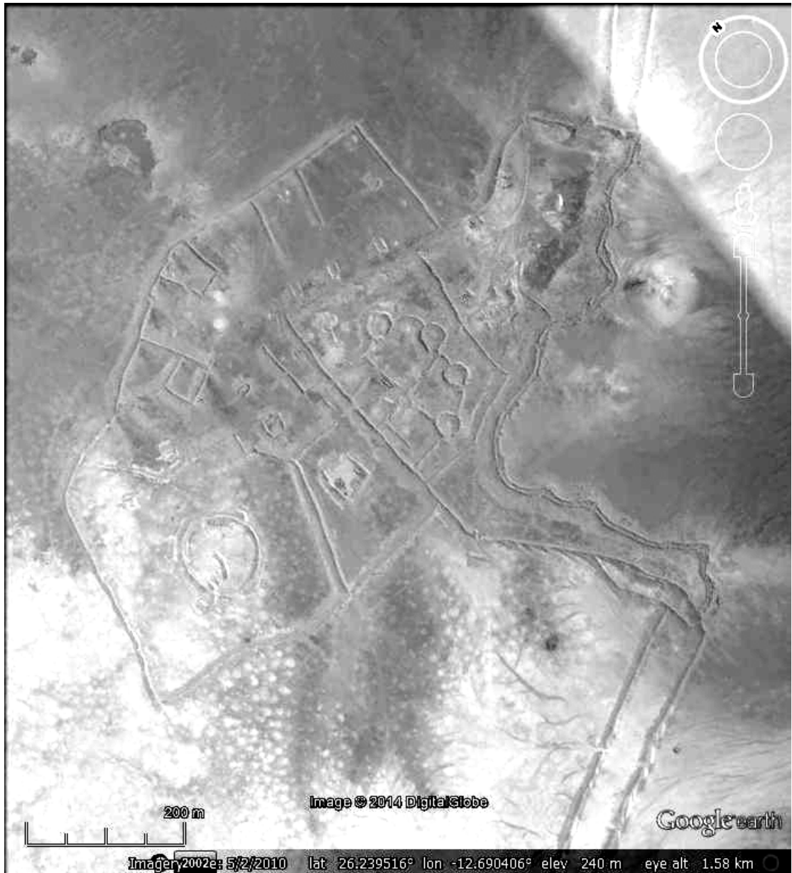
Fig. 4.66: Google Earth image (in monochrome for clarity) of ftfb 133 on Berm No. 1 (located in rectangle 187 of Fig. 4.6). This multipart installation has four gun pits located more-or-less in its centre. Probably for self propelled artillery. North is to the upper left. The scale bar in the lower left indicates 200 metres. Image date 2/5/10, DigitalGlobe.
