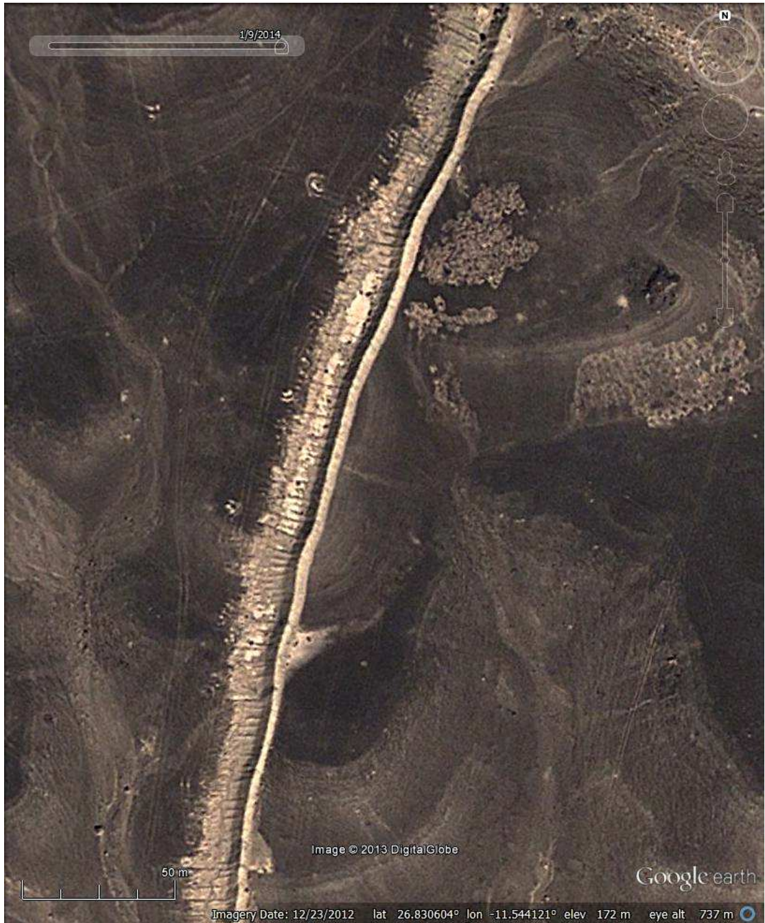
Fig. 4.29: Google Earth image along Berm No.1 (in rectangle 124 of Fig. 4.6). The bulldozer tracks are clearly visible only on the west side of the barrier. The sharply defined shadow on the west of the barrier indicates that the embankment is triangular in section. Scale bar at lower left indicates 50 metres. Image date 23/12/12, DigitalGlobe.
