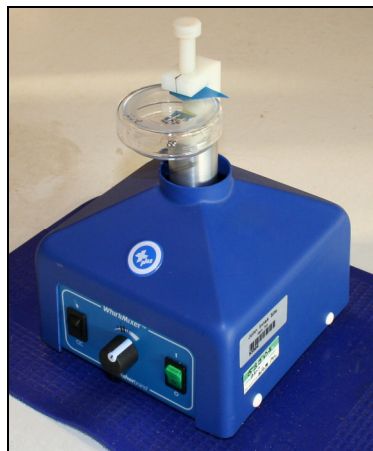
Figure 6.2: Arabidopsis Random Impact Test (ARIT) shaker
