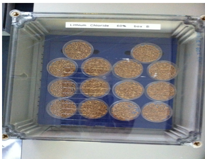
Figure 5.2. The ageing-treatment box with seeds sealed inside.
