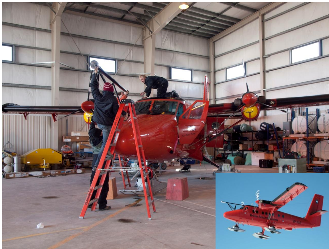
Figure 2.13: Photographs of the BAS De Havilland Canada Twin Otter aircraft in the hangar at Rothera being fitted with MASIN instrumentation and (inset, bottom right) in flight.
