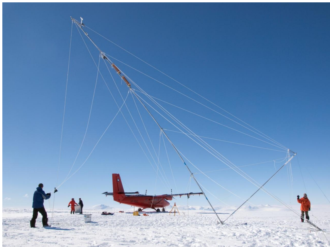
Figure 2.14: Photograph of an AWS being erected on the Avery Plateau (a high section of the AP ridge; for location see Figure 2.1c).
