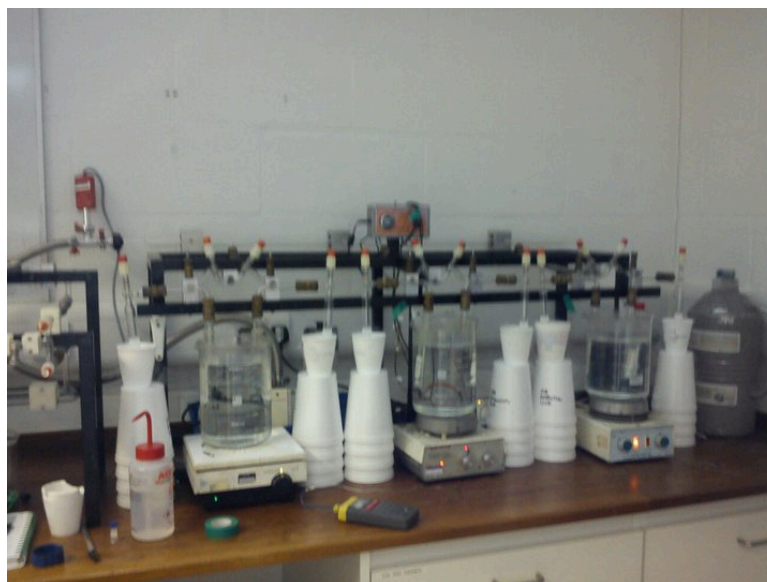
Figure 2.11: Photograph of the cryogenic vacuum distillation line set up used to extract water from leaves and xylems for hydrogen and oxygen isotope analysis, photograph (S.Newberry).
