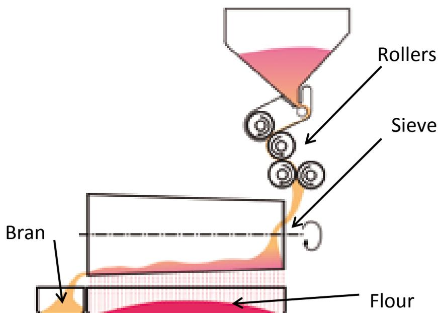
**Figure 7. Schematic of milling process in Brabender mill edited from the Brabender website (186).**
