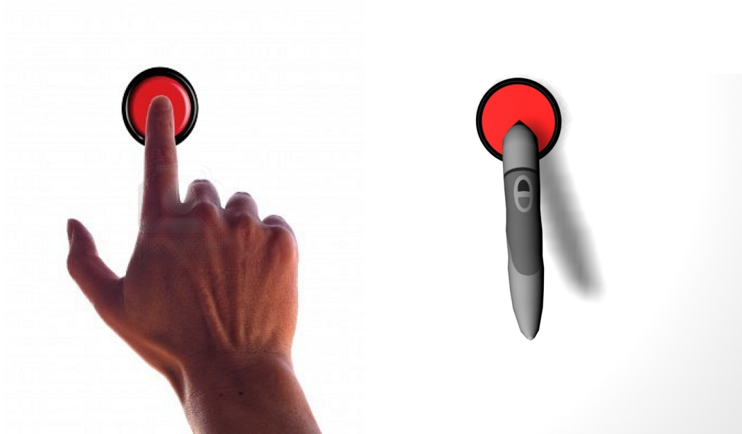
Figure 2.7: When pressing a haptic virtual switch, the operator will experience similar feedback to a tactile snap-action switch.
