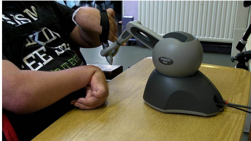
Figure 4.5: A wheelchair user operating the Phantom Omni on a height adjustable table.
