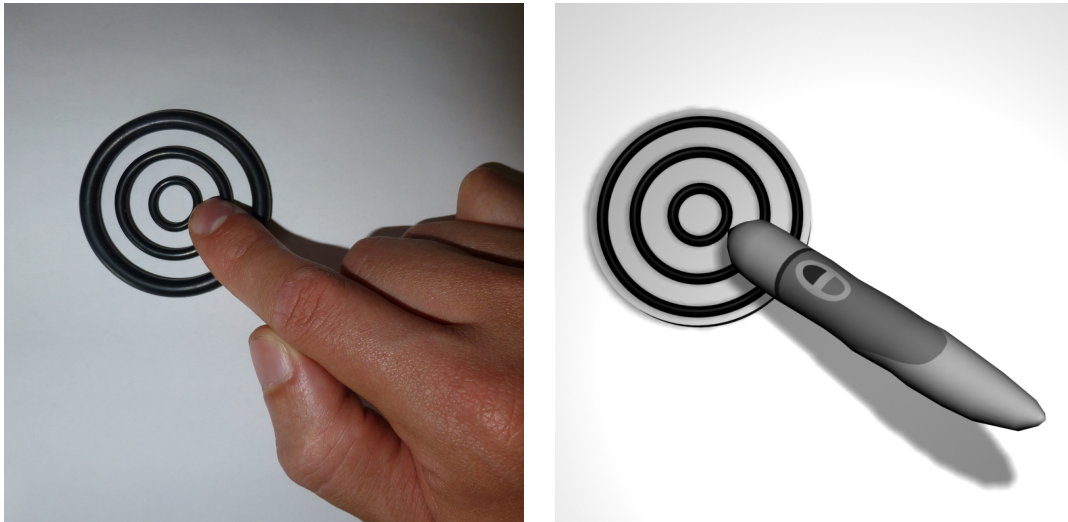
Figure 2.9: When the operator passes over surface textures, they will receive feedback from the ridges, similar to running a finger over nested O-rings.
