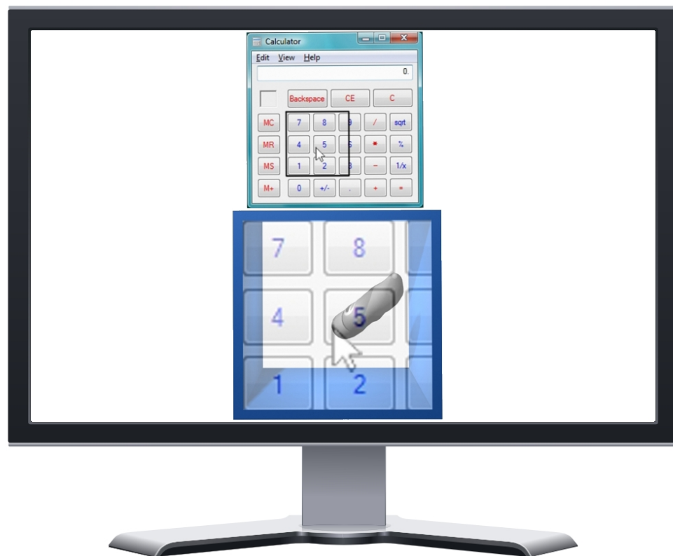
Figure 3.25: The black square surrounding the cursor indicates an area of the screen that will be magnified in the haptic workspace and screen space. The magnified semi-transparent window is overlaid on top of the workbook.
