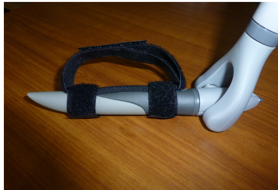
Figure 5.26: The adjustable strap designed for the Phantom Omni to assist with grasping the stylus.
