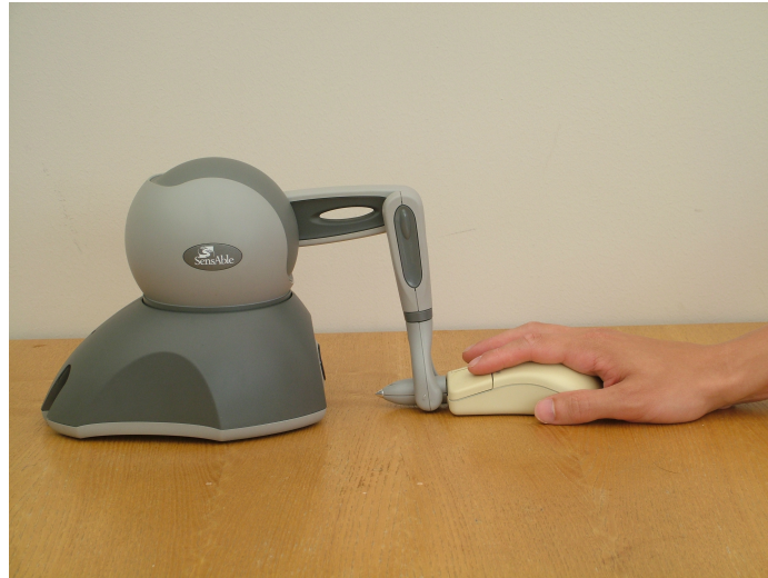
Figure 6.1: The concept of using the Phantom Omni in a mouse configuration.
