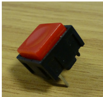
Figure 3.6: The snap-action tactile switch used for device switching operations.
