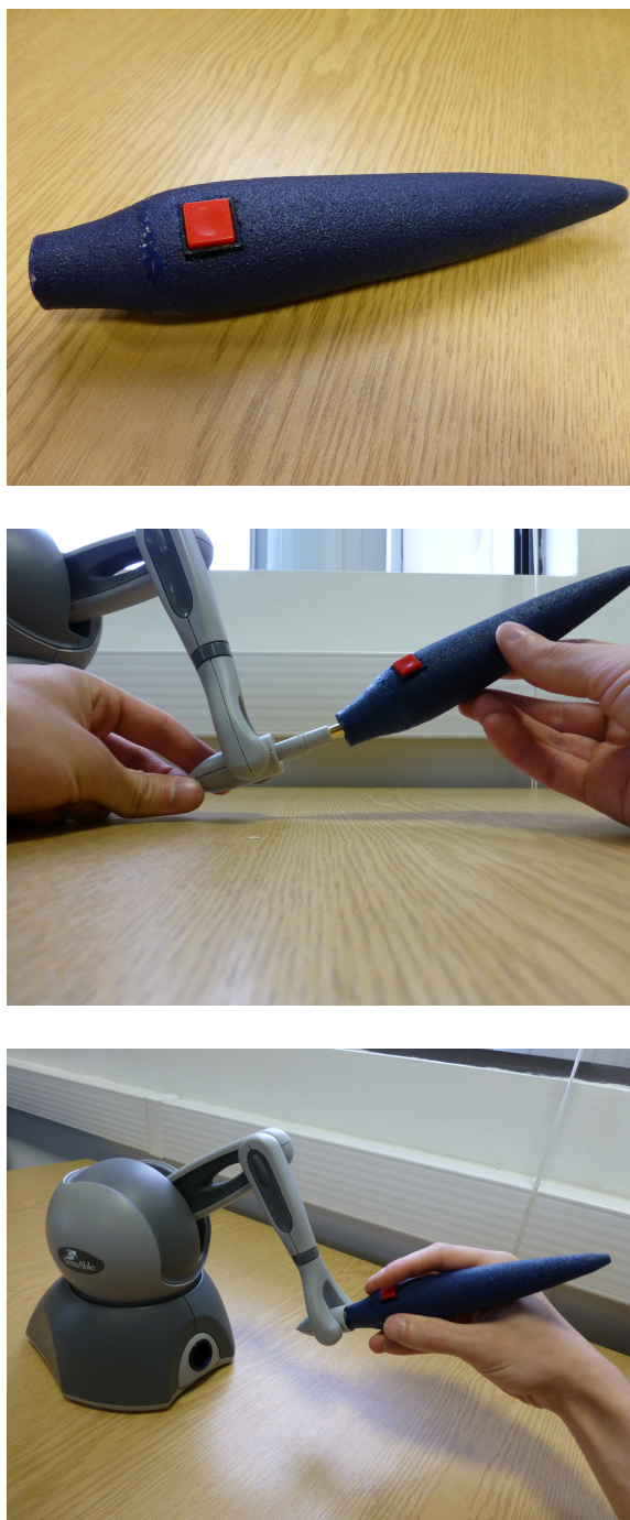
Figure 3.8: Mounting the finished device handle to the Phantom Omni.
