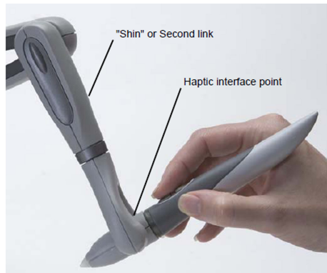
Figure 1.2: The HIP position on the Phantom Omni (adapted from Openhaptics Toolkit Programmer's Guide [OHT14]).
