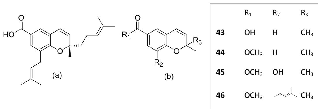
Figure 1.9 - Structures of chromenes isolated from (a) *Piper gaudichaudianum* and (b, **43** - **46**) *P. Aduncum*
