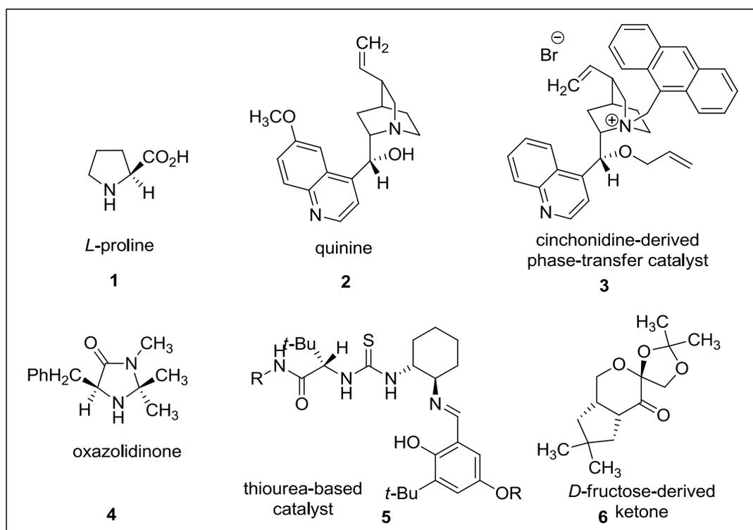
Figure 1.1 - Some typical organocatalysts
