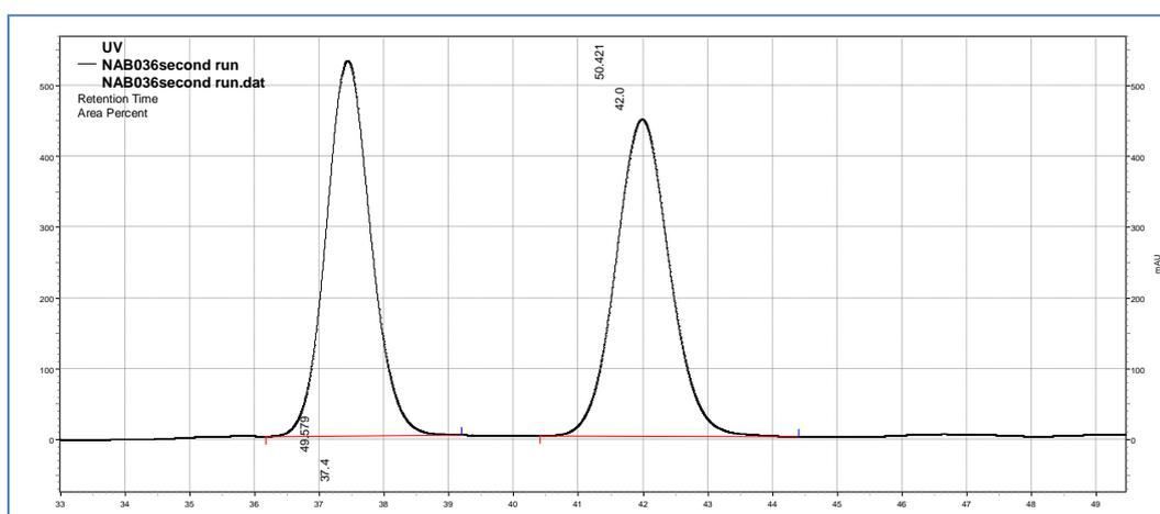
Figure 2.19 - HPLC trace of the racemic epoxide **124**
