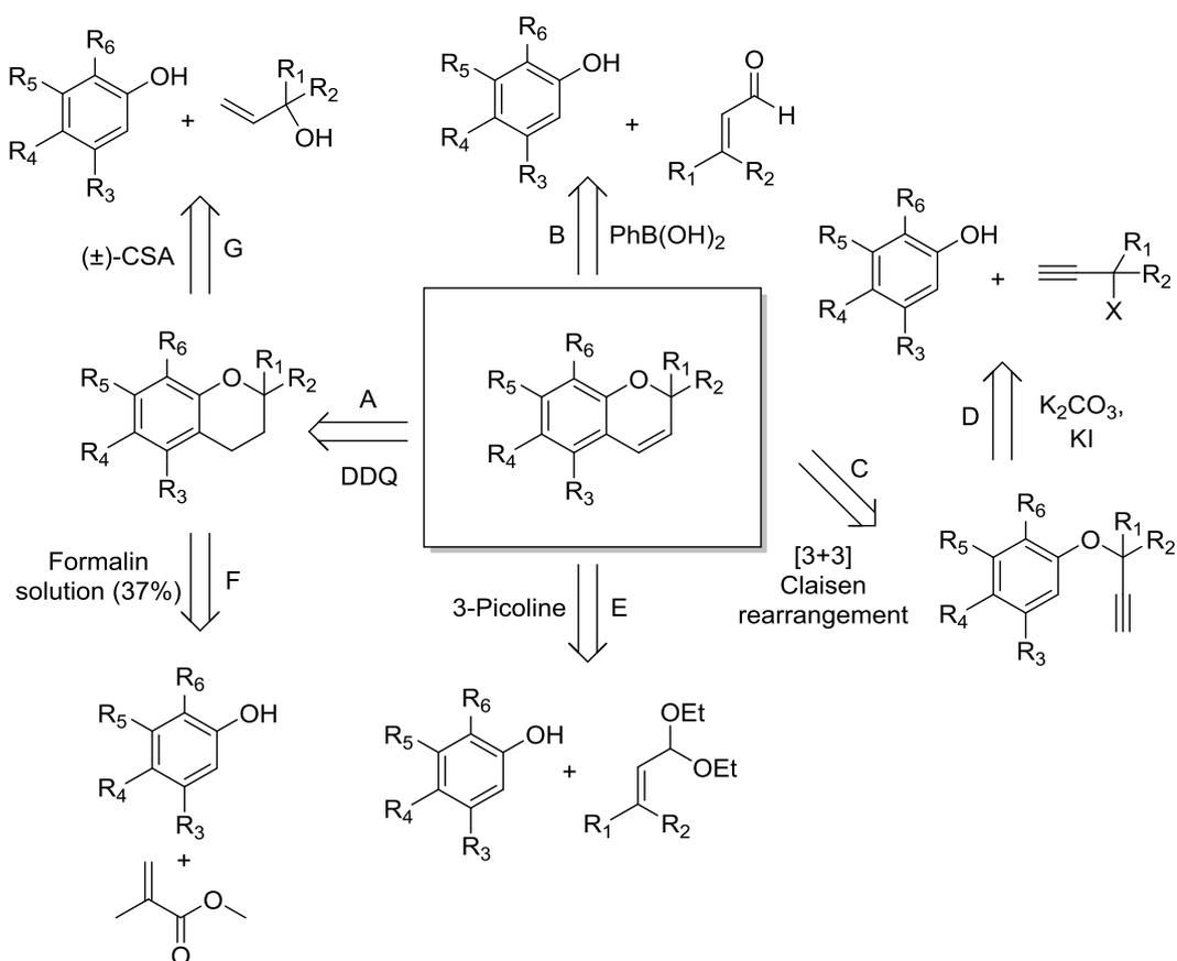
Figure 2.27 - Various synthetic approaches for the synthesis of chromenes **47** – **50**
