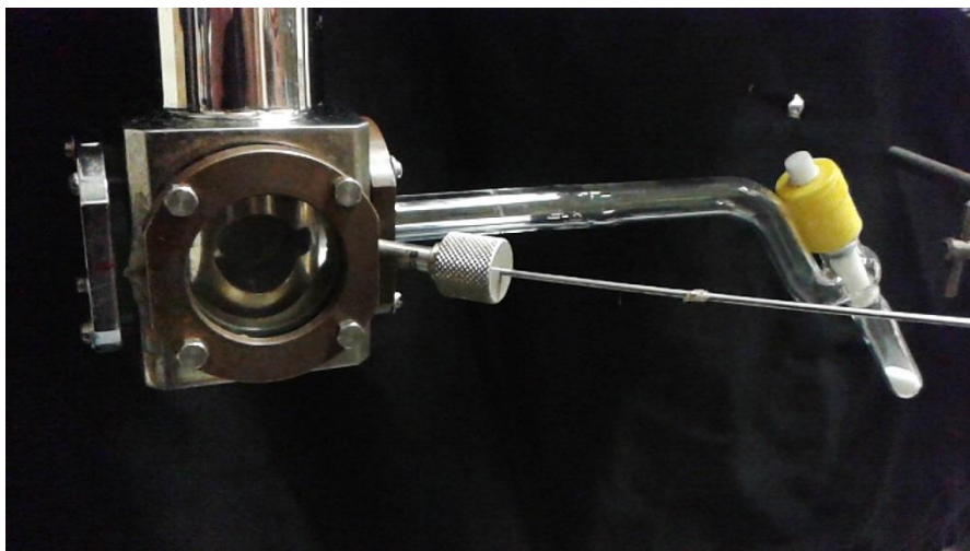
Figures 1-6a, b and c: Orientation of temperature controlled glassware relative to Sample Chamber G showing relation of CsI window to incoming argon gas stream (greyed out) from needle H versus normal sample scanning orientation (solid line), detail view of glassware construction showing heating elements and insulation; photograph of glassware relative to sample chamber.
