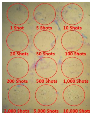
Figure 87 Durability test to ensure the CD could withstand the LASER
