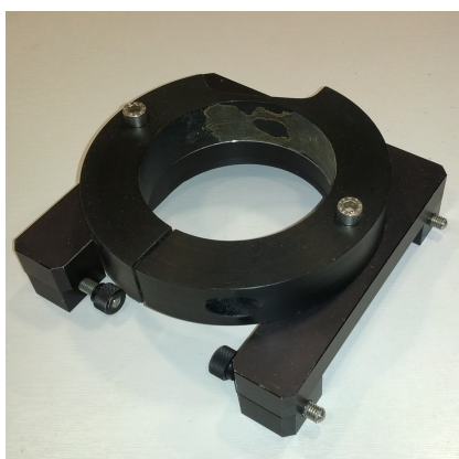
(c) Oxford flow cryostat with cryostat removed
