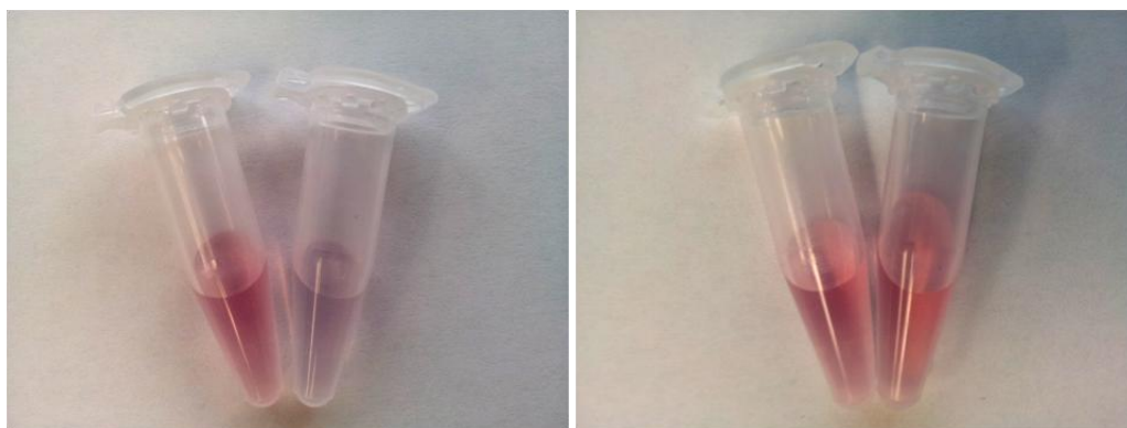
Figure 86 Solutions of gold nanoparticles containing 2mM bisacridine 2. A change from red to colourless corresponding to the change in peak position in Figure 84 is shown (left) alongside the same solution after the addition of 12 \mu l of 20 mM SDS (right). In each case, the left hand eppendorf contains a solution of gold nanoparticles and DNA.
