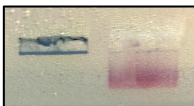
Figure 105 Agarose gel comparing the electrophoretic character of a solution of gold citrate nanoparticles (left lane) and a solution of the same nanoparticles functionalised with DNA (right lane). The blue colour apparent in the left lane is typical of precipitated gold nanoparticles. The stability of the functionalised nanoparticles under these conditions confirms the attachment of the DNA.
