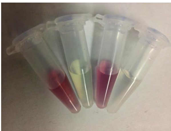
Figure 80 Solutions of gold nanoparticles. From left, control (no ligand), 10 mM bisacridine 2, 20 mM 9-aminoacridine, 10 mM bisacridine 3. The colour change from red to colourless is typical of gold nanoparticle aggregation caused by the bisacridines.
