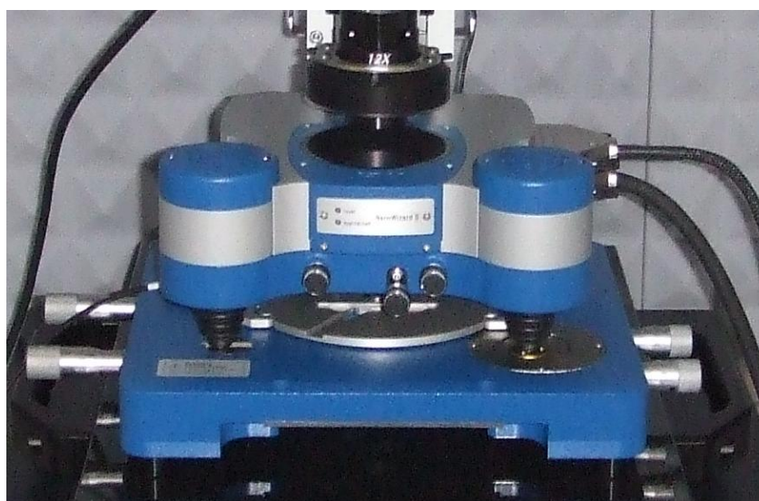
Figure 19 A Photograph of a JPK NanoWizard II™ atomic force microscope. Visible, from top to bottom, are the optical microscope, AFM scanning head, and the sample stage.
