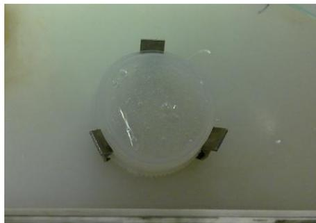
**Figure 2.26** Plastic gel sample holder for dissolution test equipped with a metal plate and filled with gel with 60% water.
