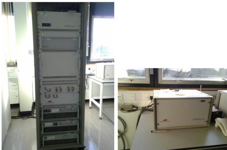
**Figure 2.23** 23.4 MHz NMR (Maran Ultra) interfaced to a DRX console (on the left)
