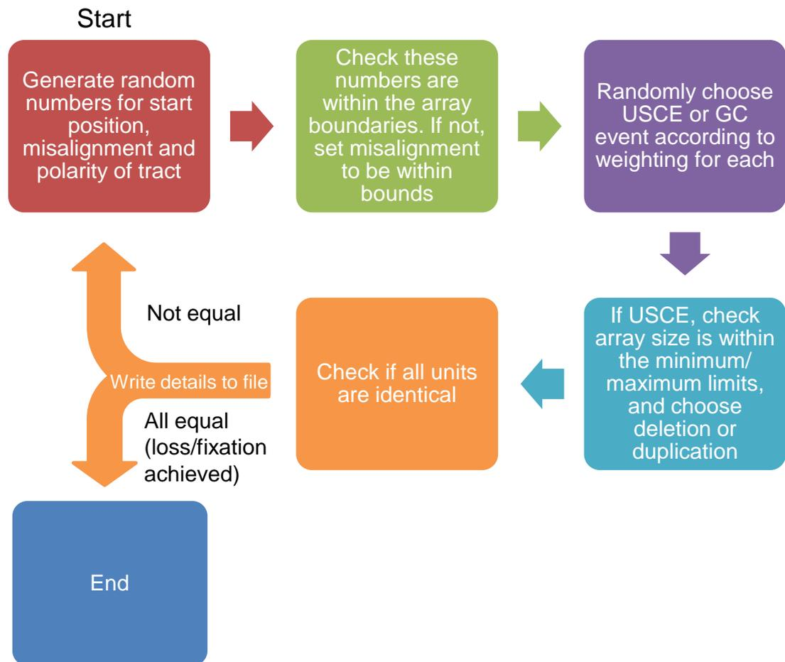
Figure 4.2.: Overview of each iteration of a simulation in the SIMPLEX program
