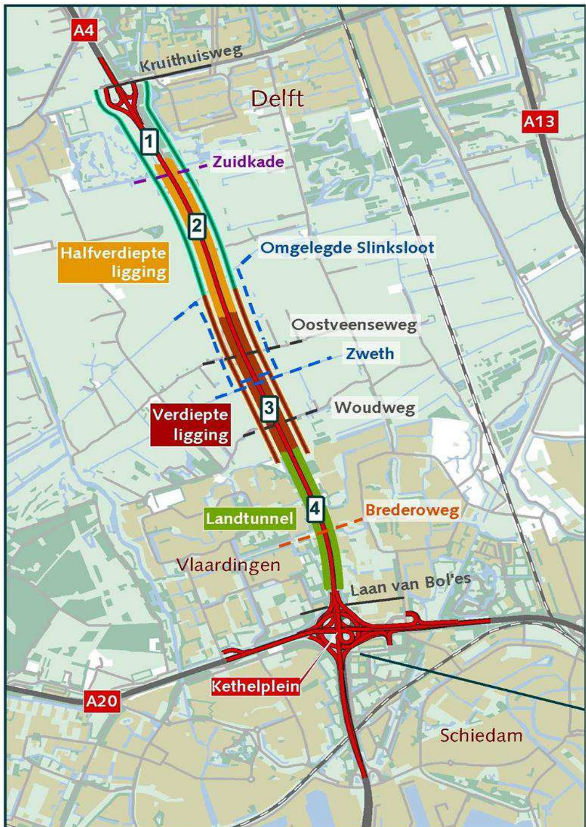
Map 4.4: Overview of the A4DS and the impact area (Rijkswaterstaat, 2009d). Terms of reference: (2) = in half-deep cuttings ('halfverdiepte ligging'); (3) = in deep cuttings ('verdiepte ligging'); (4) = land tunnel
