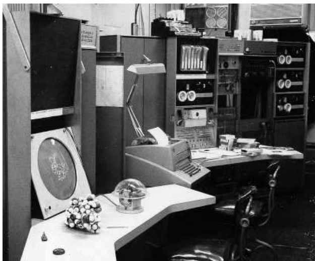
Figure 2.1: Overview of the molecular modelling system, with the KLUGE in the lower left corner, and a space-filling model by the display. Photo courtesy of Martin Zwick.
