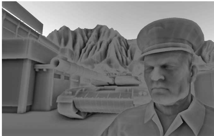
Figure 2.10: Resulting image from Mittring's implementation of SSAO [Mit07]. Incorrect shading of geometry is clearly visible due to over occlusion, resulting in an overly dark image. This is corrected in later implementations.
