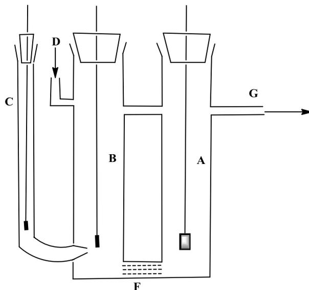
**Figure 1.2** Electrochemical cell A counter electrode, B working electrode, C reference electrode, D, G inlet and outlet taps for purging gas, F a frit for ion exchange.
