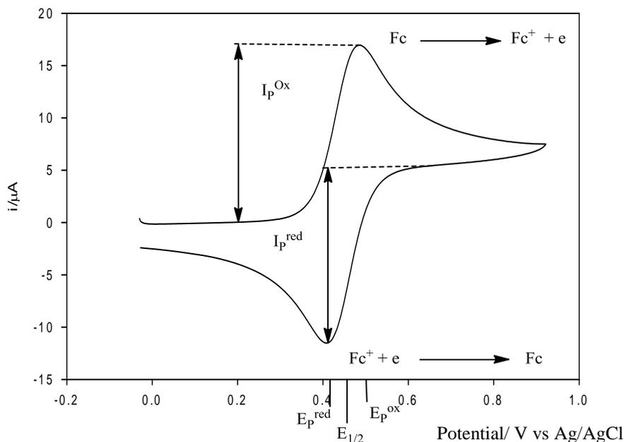
**Figure 1.4** Cyclic voltammogram of a solution of ferrocene in 1.5 mM  $\text{CH}_3\text{CN}/[\text{NBu}_4][\text{BF}_4]$  at carbon electrode, scan rate  $\nu = 0.025 \text{ V s}^{-1}$ .
