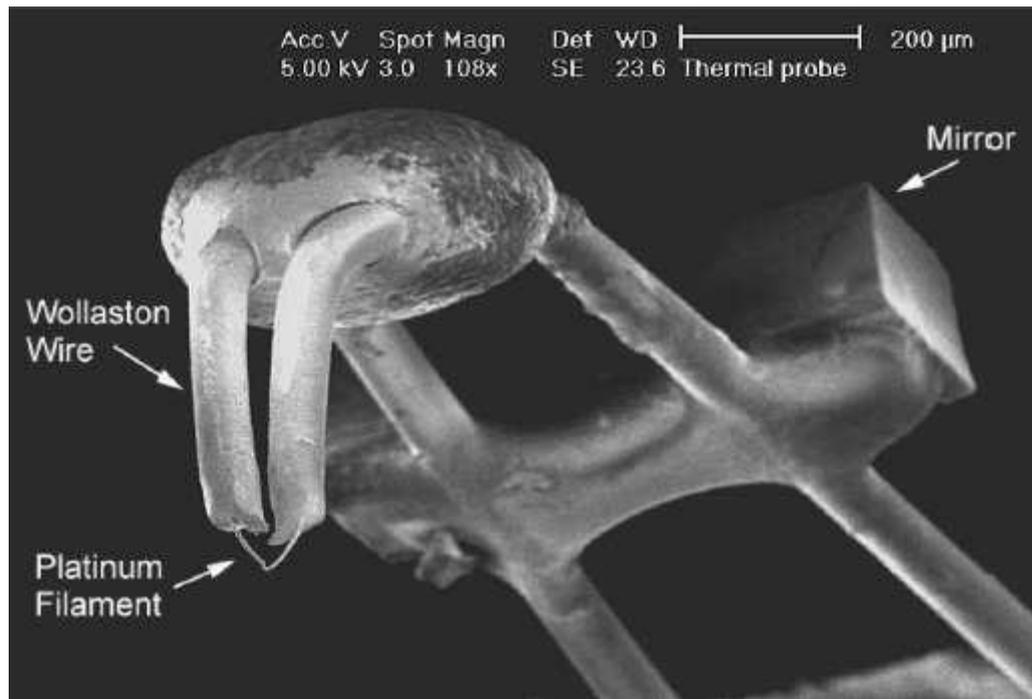
Figure 2.6 A Wollaston wire probe (reproduced from Royall *et al.*, 2001b)
