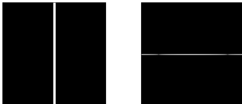
Fig C10 The Fourier transforms from adding an infinite range of harmonic frequencies
