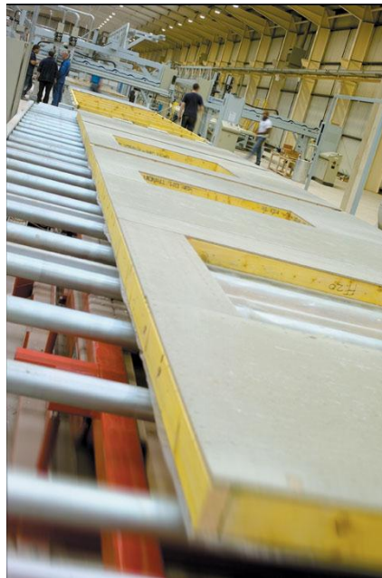
Figure 1-12: Factory production of panel system (image source: Space4)
