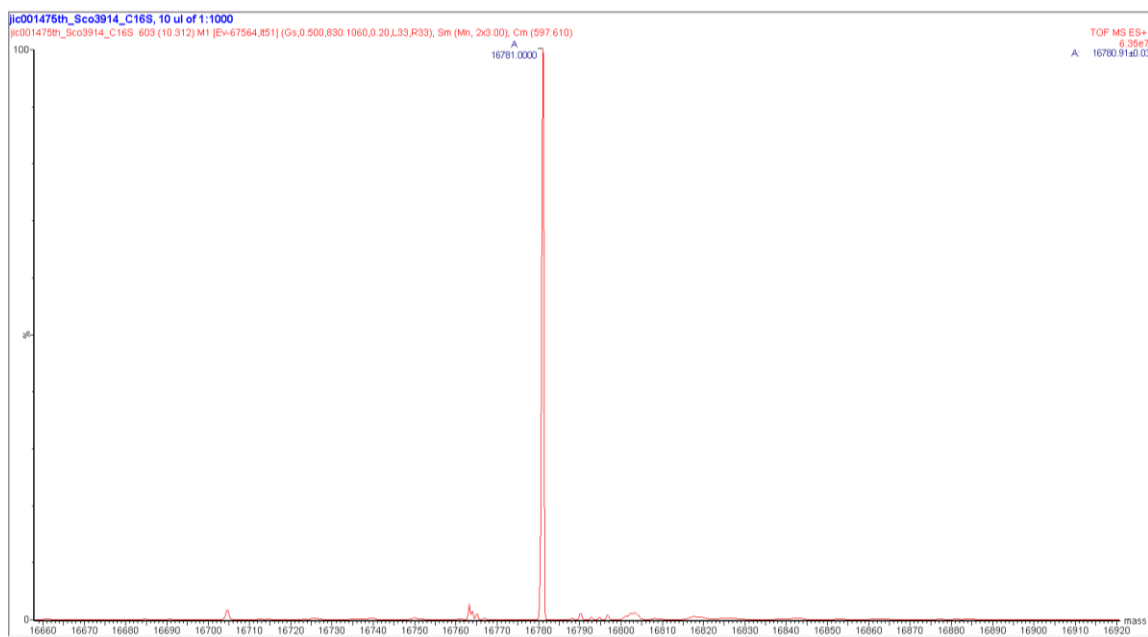
Figure 3.28 Intact mass analysis of Sco3914C16S. The main peak indicates that the protein has a molecular weight of 16781 Da \pm 0.03. This corresponds to a difference of +76 Da from the expected molecular weight of the protein which is 16705 Da.
