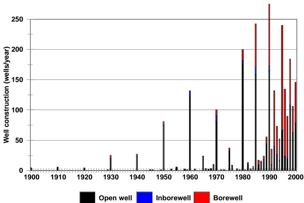
Figures 20 and 21 present the number of wells of different types constructed during the 20<sup>th</sup> Century in Kalyandurg and Dhone respectively. As information on date of construction of wells was elicited in part from local villagers, information for the first part of the century is presented on a decadal basis. The peaks in well construction during the first part
