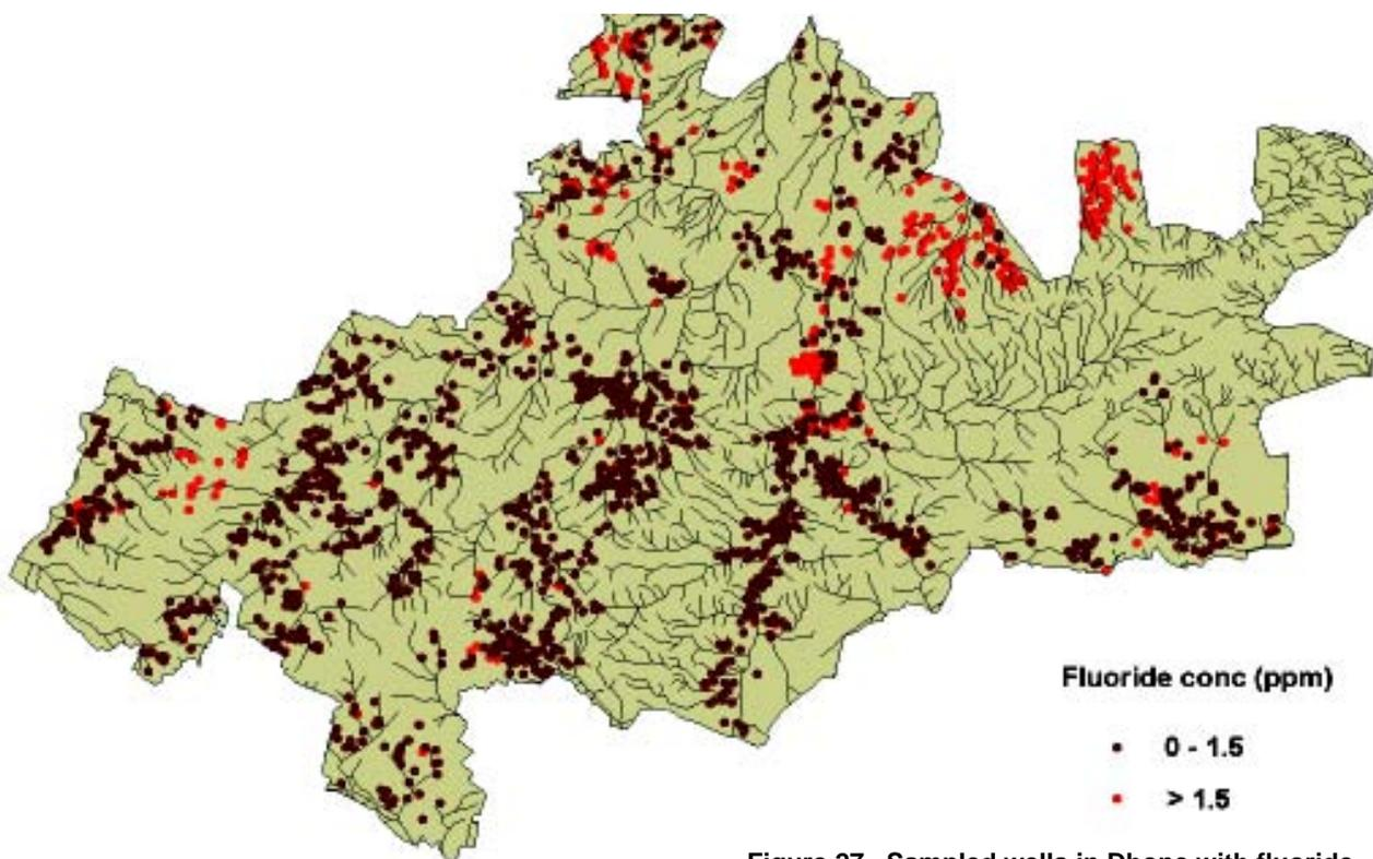
**Figure 27. Sampled wells in Dhone with fluoride exceeding domestic water permissible limits**
