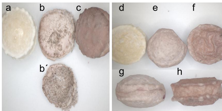
Figure 6.16 Optical microscopy images of paracetamol tablets coated (TWG = 20%) with 1:5 HAS/Zein after 24 hours immersion in phosphate buffer pH 6.8 (a), Protocol II colonic (b, b', where b and b' represent the two halves of the ruptured coating) and Protocol II control (c) conditions. Images d, e and f are paracetamol tablets coated (TWG = 20%) with zein alone pseudolatex after 24 hours immersion in the same conditions as a to c. Images g and h are profile views of tablets coated with zein alone pseudolatex after 24 hours immersion in Protocol II control (g) and phosphate buffer (h) conditions.
