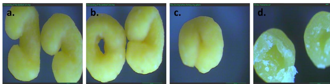
Figure 3.2 Microscopic images (4x) that represent the suggested mechanism of sphere formation during the spheronization step. The mechanism starts with: (a) partially folded extrudates, (b) doughnut-shaped units, (c) sphere, and (d) cross-section of a pellet showing a cavity.
