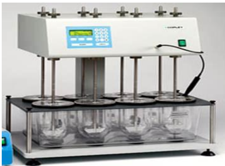
Figure 2.4 A photograph showing the dissolution bath used to conduct the dissolution tests presented in this work (D8000, Copley Scientific Ltd.).
