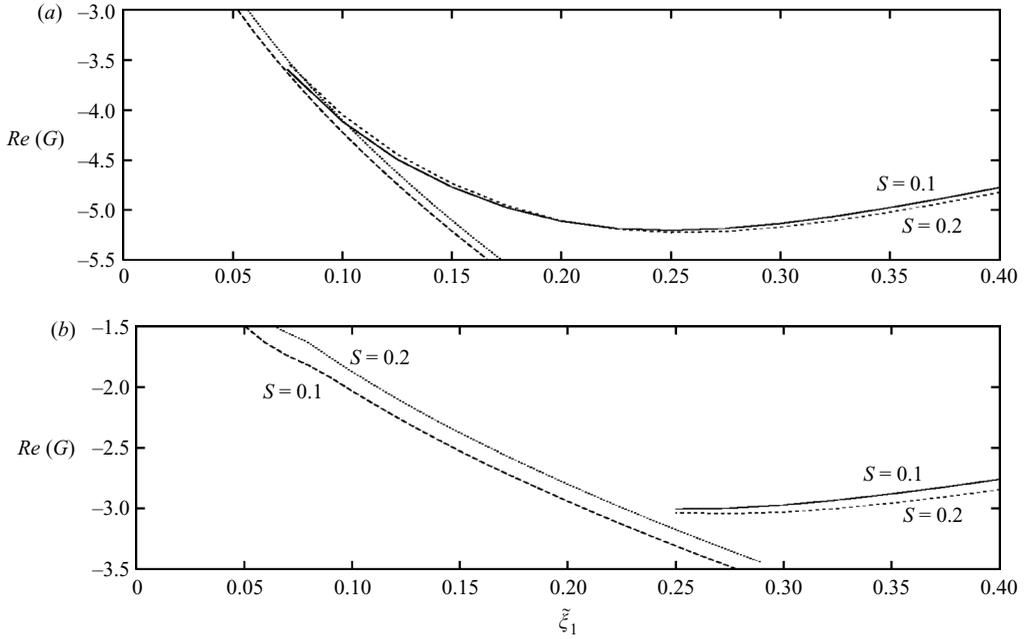
FIGURE 2. Plot of the real part of the growth rate  $G(\xi_1)$  as a function of downstream distance  $\xi_1 = 2\epsilon^2 \xi_R / U_0^2$ , calculated by the leading edge receptivity analysis and local PSE theory, for  $S = 0.1$  and  $S = 0.2$  for the cases (a)  $\epsilon = 0.05$  and (b)  $\epsilon = 0.1$ .
