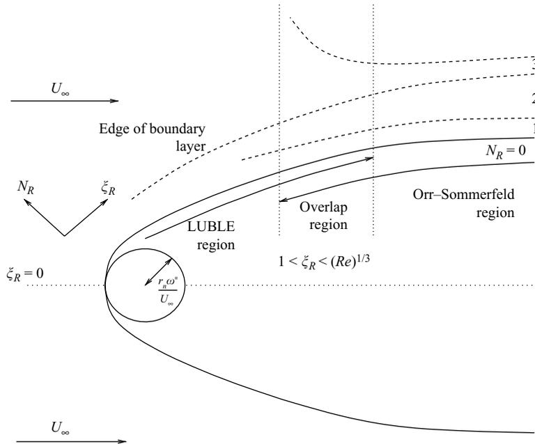
FIGURE 1. Illustration of the boundary layer structure for a general body with dimensional nose radius  $r_n$  at zero angle of attack to the mean flow. The three-deck asymptotic structure in the Orr–Sommerfeld region consists of: 1, the viscous wall layer; 2, the main inviscid layer; 3, the outer irrotational layer.
