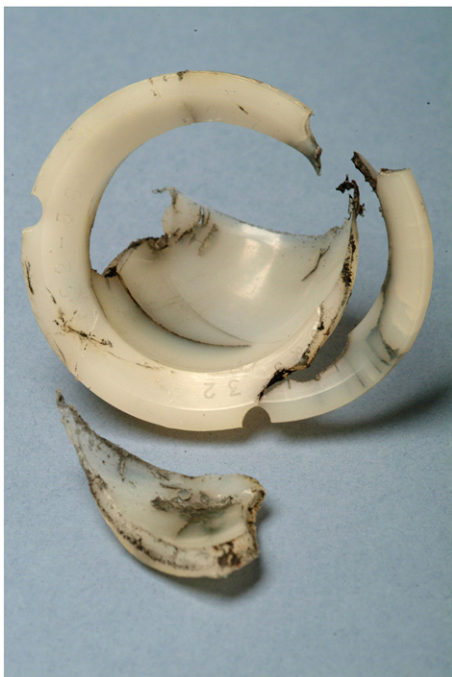
Fig. 4. Fractured polyethylene liner removed from socket.
