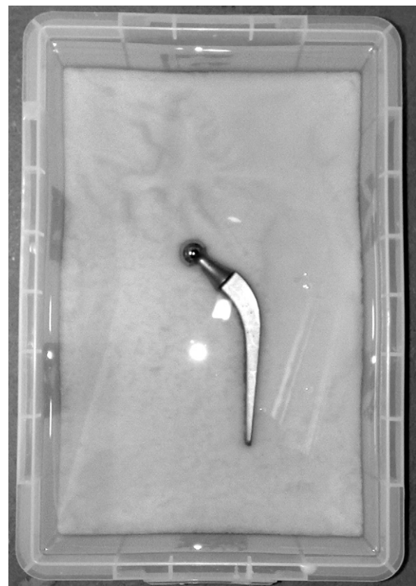
Figure 1 Hip prosthesis phantom made from a Charnley femoral component set in 8 kg of solid vegetable fat.
