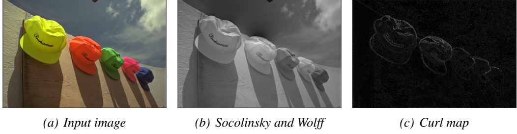
Figure 5.2: An example of image (from the dataset by Kodak, 2004) whose colour tensor gradient field is non-integrable: the Fourier integration yields an output image with a dark halo by the second hat from the left. In (c) we visualise the curl of the colour tensor gradient (darker is smaller, lighter is larger). We notice that the most visible artefacts appear where the curl is large for many pixels.
