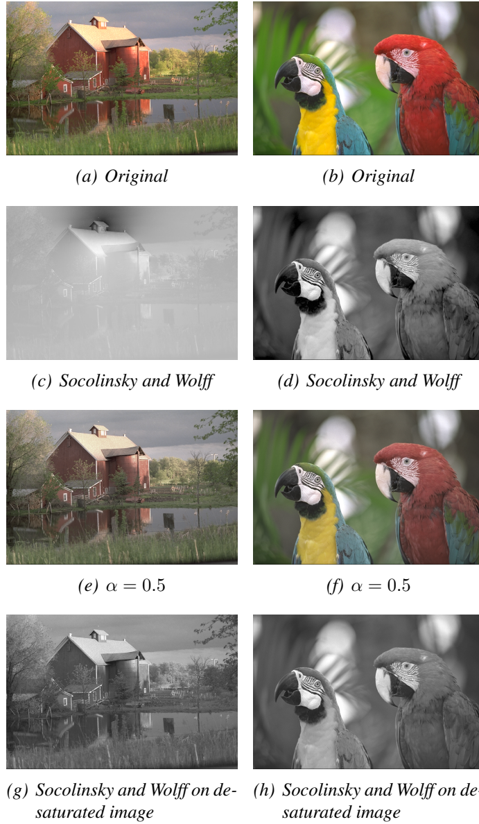
Figure 5.6: Images from the Kodak dataset (Kodak, 2004) processed with Socolinsky and Wolff’s technique before and after desaturation. Note the heavy integrability artefact in (c), completely removed in (g) by means of the desaturation. However, the image in (d) is artefact-free and the desaturation, in this case, only reduces the contrast (h). This phenomenon is not observed in (c) and (g) because the artefact is well out of the range [0, 1] . Thus, the linear global mapping makes the rest of the image look “washed out”.
