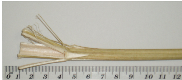
Figure 5.2: Hemp stem. The two stem components, fibre and shiv, can be seen at the frayed end of the stem.
