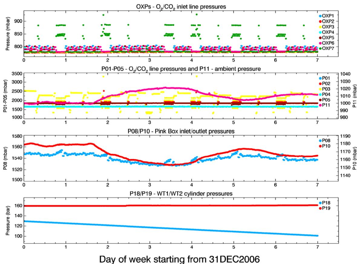
**Fig. 2.** Example of diagnostic parameters, showing all pressures relevant to the O<sub>2</sub> and CO<sub>2</sub> system over a one-week period starting from 31 December 2006. Each data point in the figure is a 16 min average (for all parameters). The labels in the legends correspond with those shown in Fig. 1.
