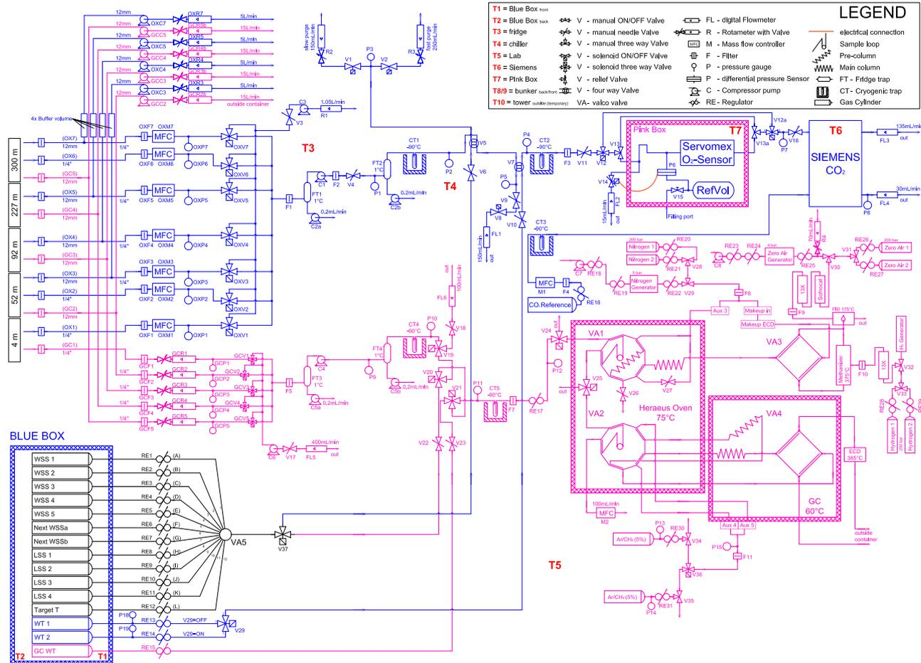
**Fig. 1.** Gas-handling schematic for atmospheric measurements of O<sub>2</sub> and CO<sub>2</sub> (shown in blue), and CH<sub>4</sub>, CO and N<sub>2</sub>O (shown in pink). As schematically represented, there appear to be dead volumes downstream of 3-way valves OXV1-7 and GCV1-5, however, in reality they are mounted in a manifold arrangement with zero dead volume.
